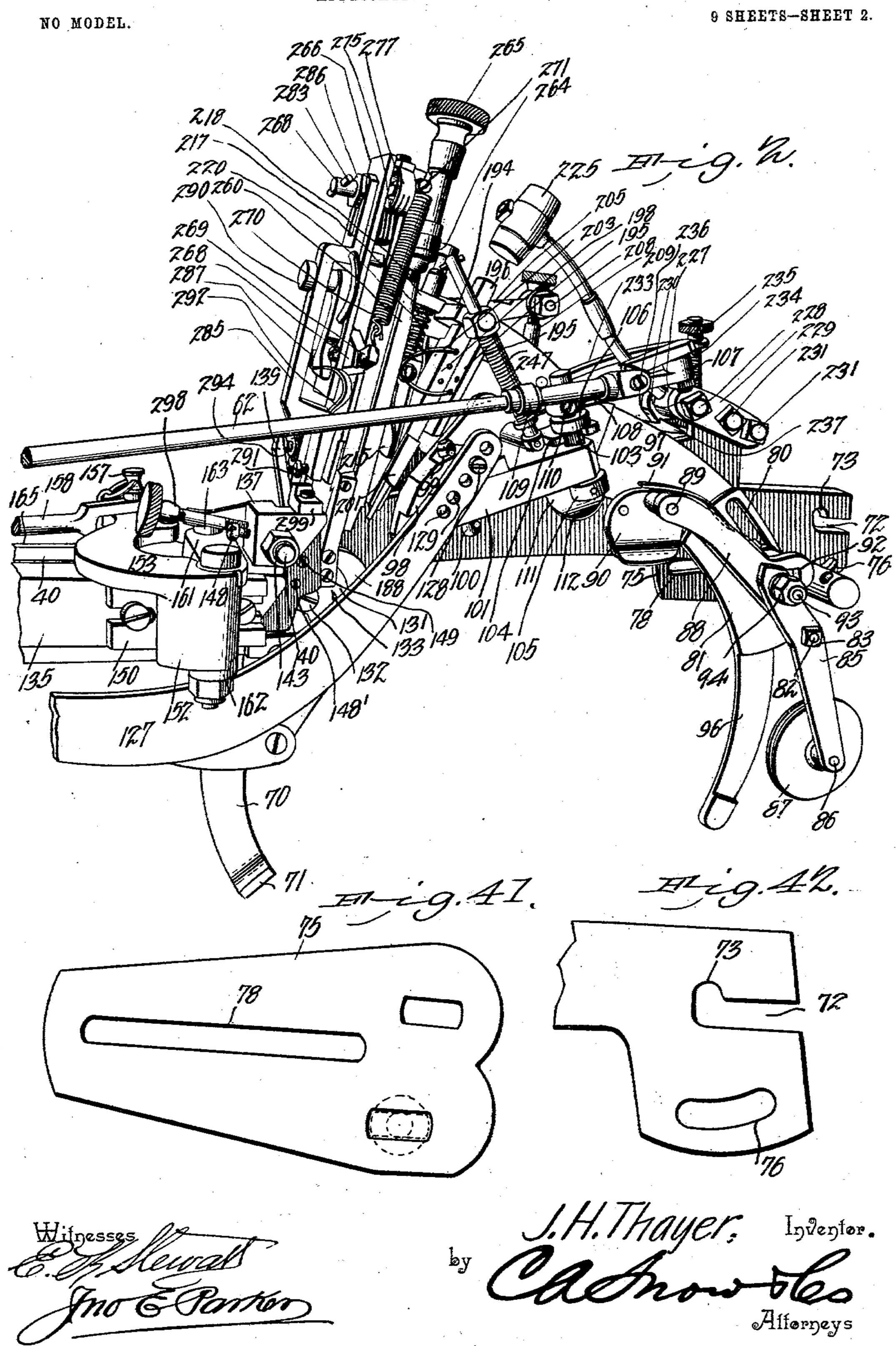
MACHINE FOR GUMMING AND STRAIGHTENING THE TEETH OF SAWS.
