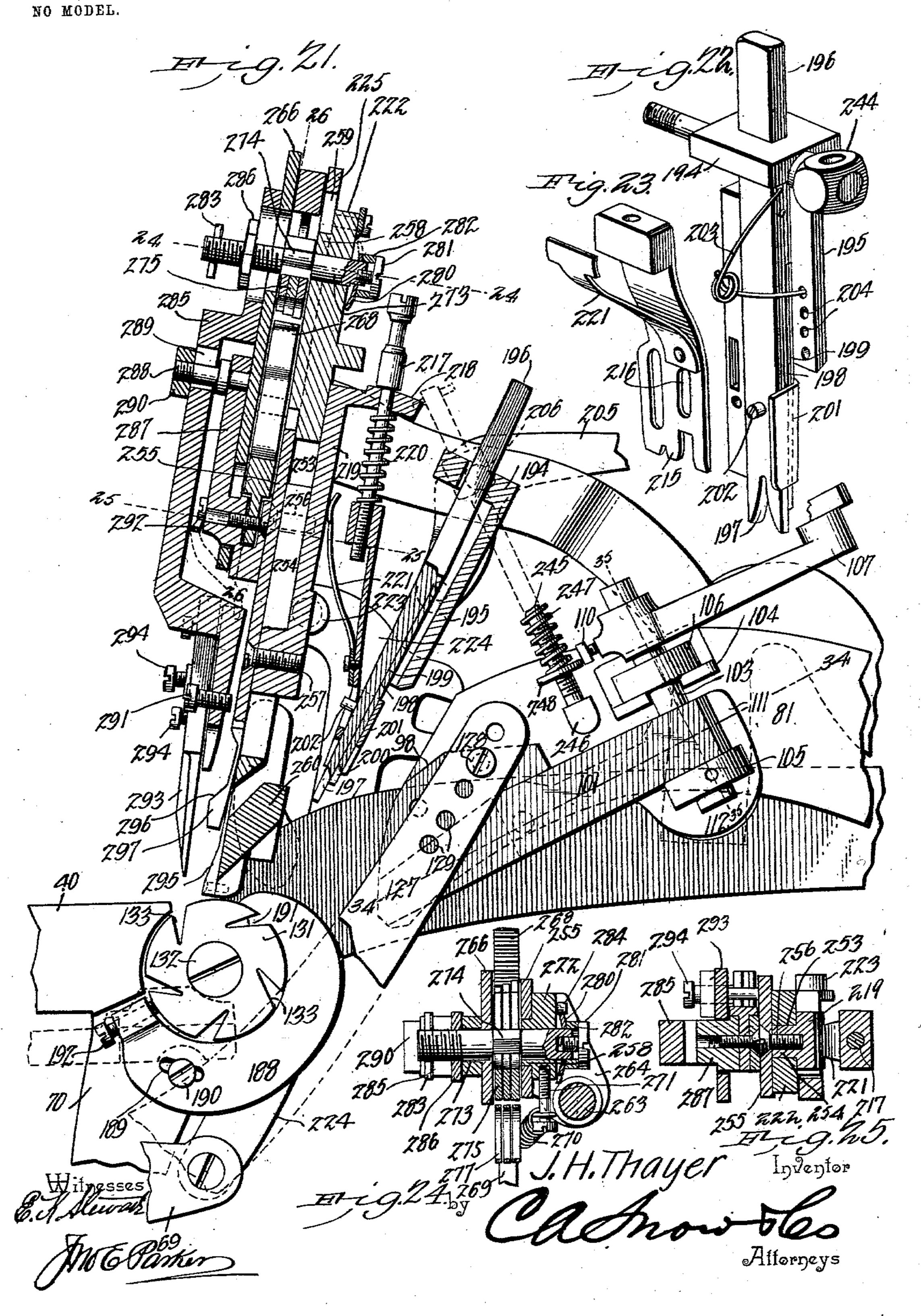
MACHINE FOR GUMMING AND STRAIGHTENING THE TEETH OF SAWS.
