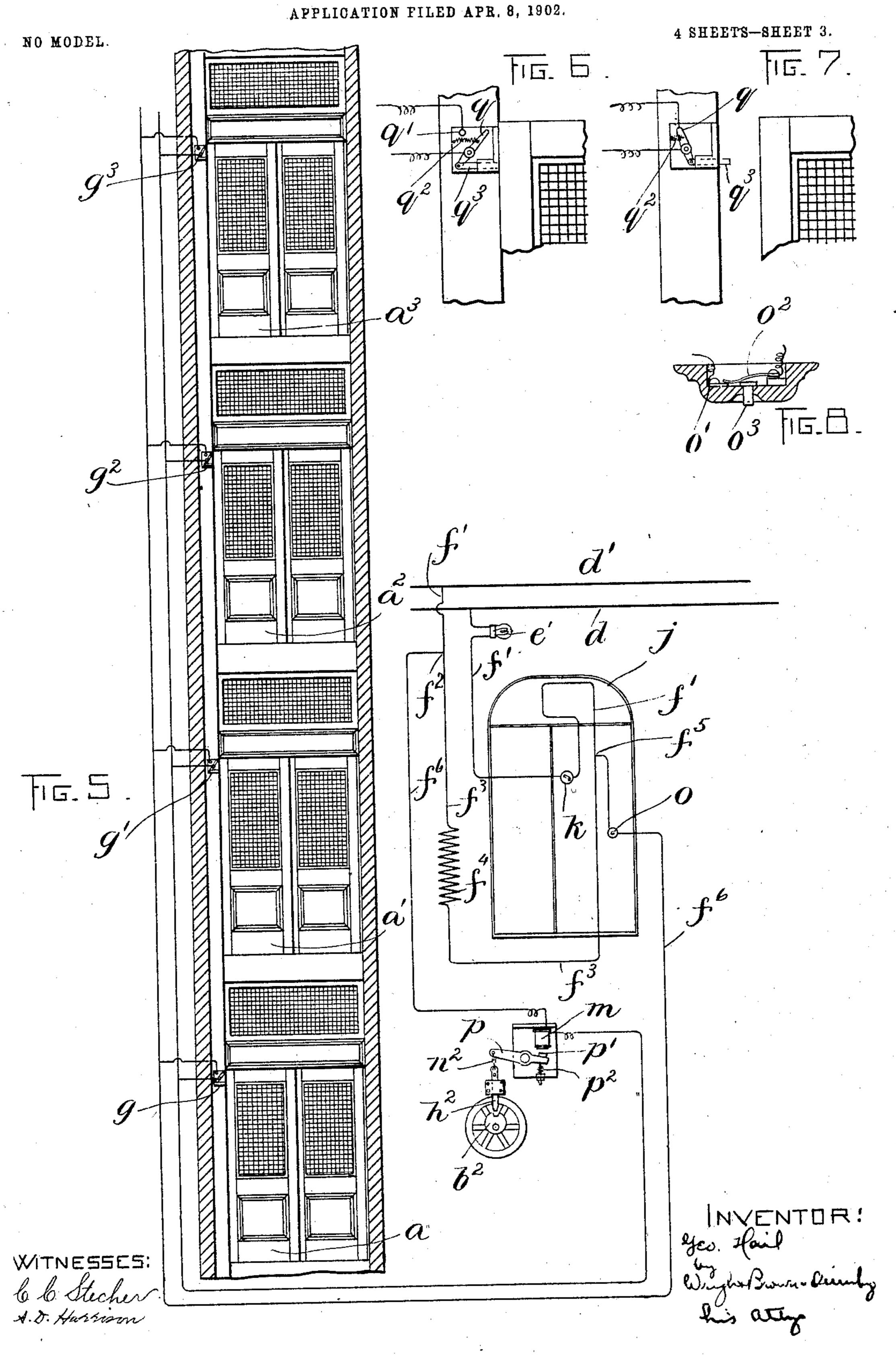
G. HAIL. ELECTRIC SYSTEM FOR ELEVATOR SAFETY APPLIANCES.
