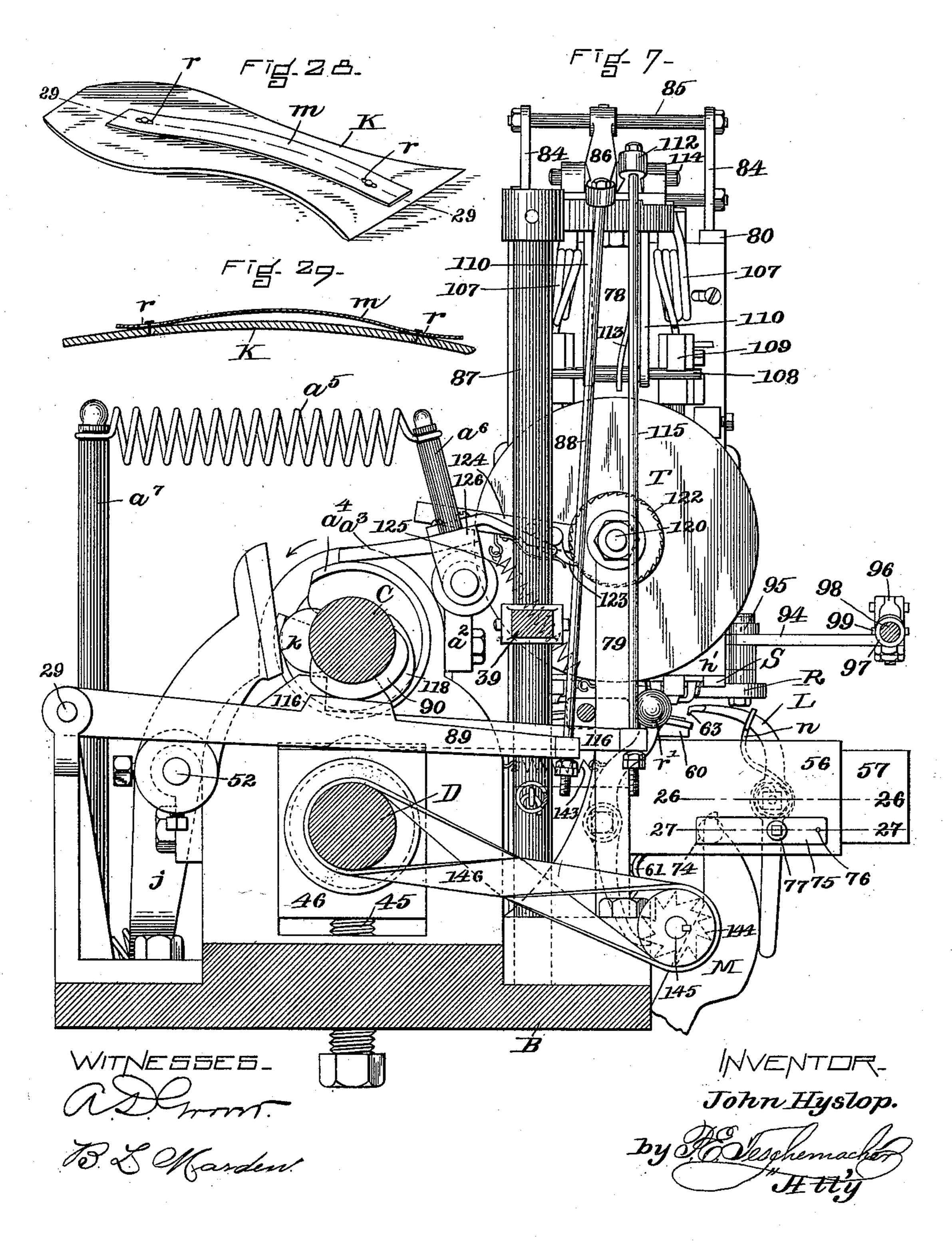
MACHINE FOR MAKING LEATHER BOARD BOOT OR SHOE SHANKS, &c No. 591,353. Patented Oct. 5, 1897.
