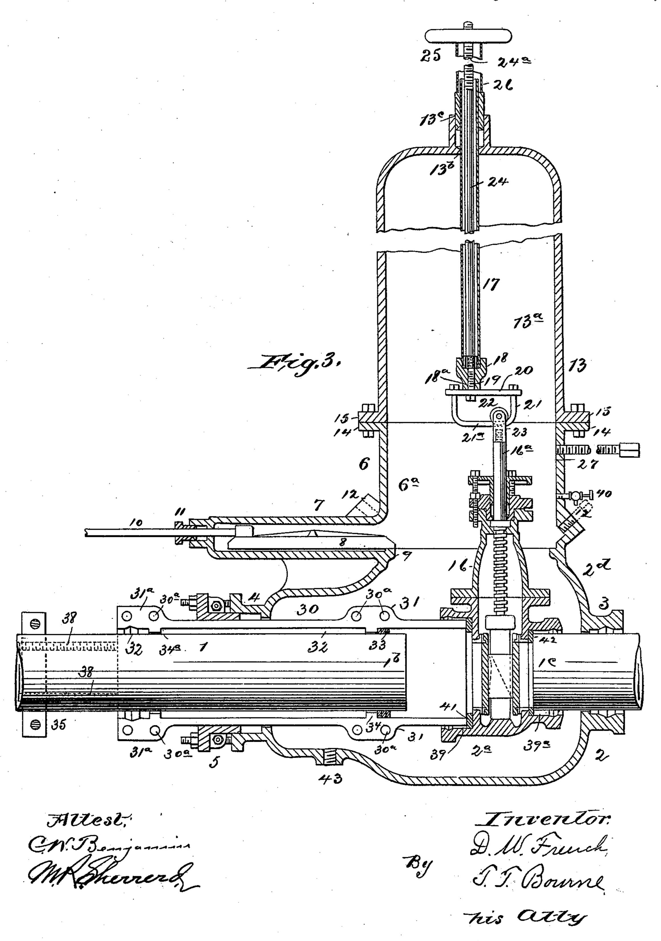
MEANS FOR INSERTING VALVES IN PIPES OR MAINS.
