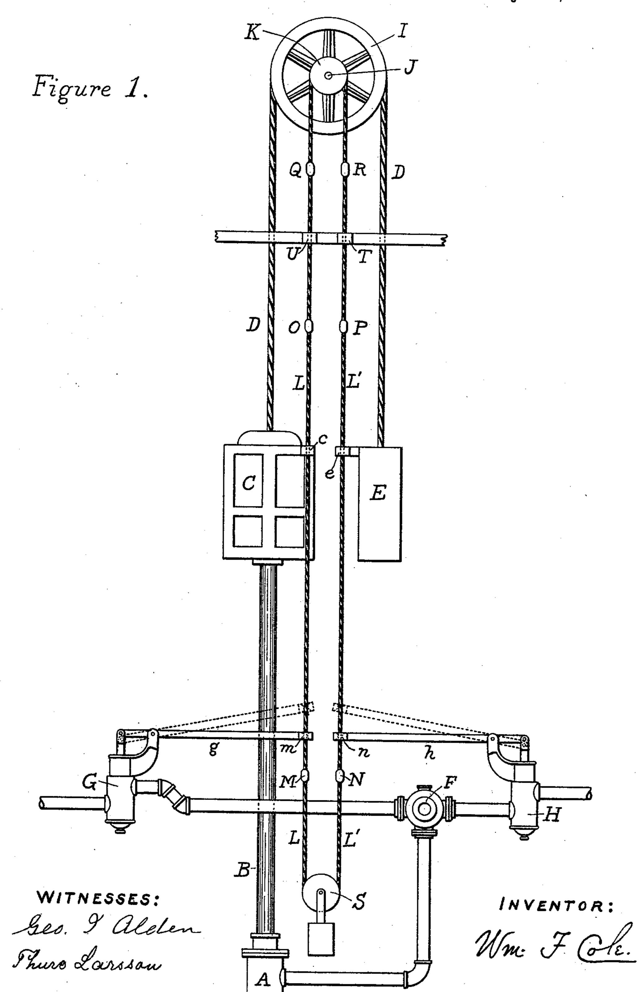
MECHANISM FOR OPERATING VALVES OF HYDRAULIC ELEVATORS.
