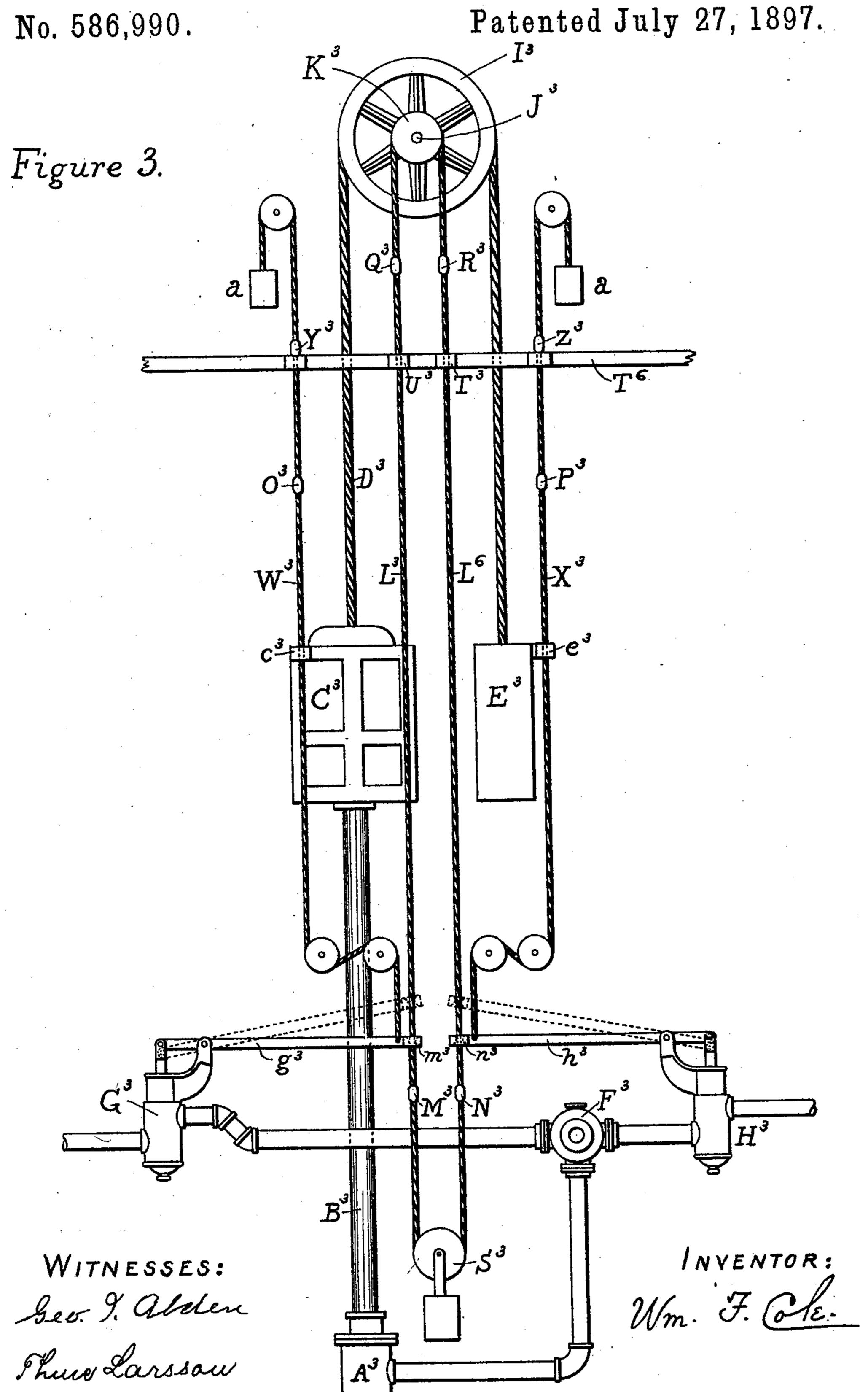
MECHANISM FOR OPERATING VALVES OF HYDRAULIC ELEVATORS. No. 586,990. Patented July 27, 1897.
