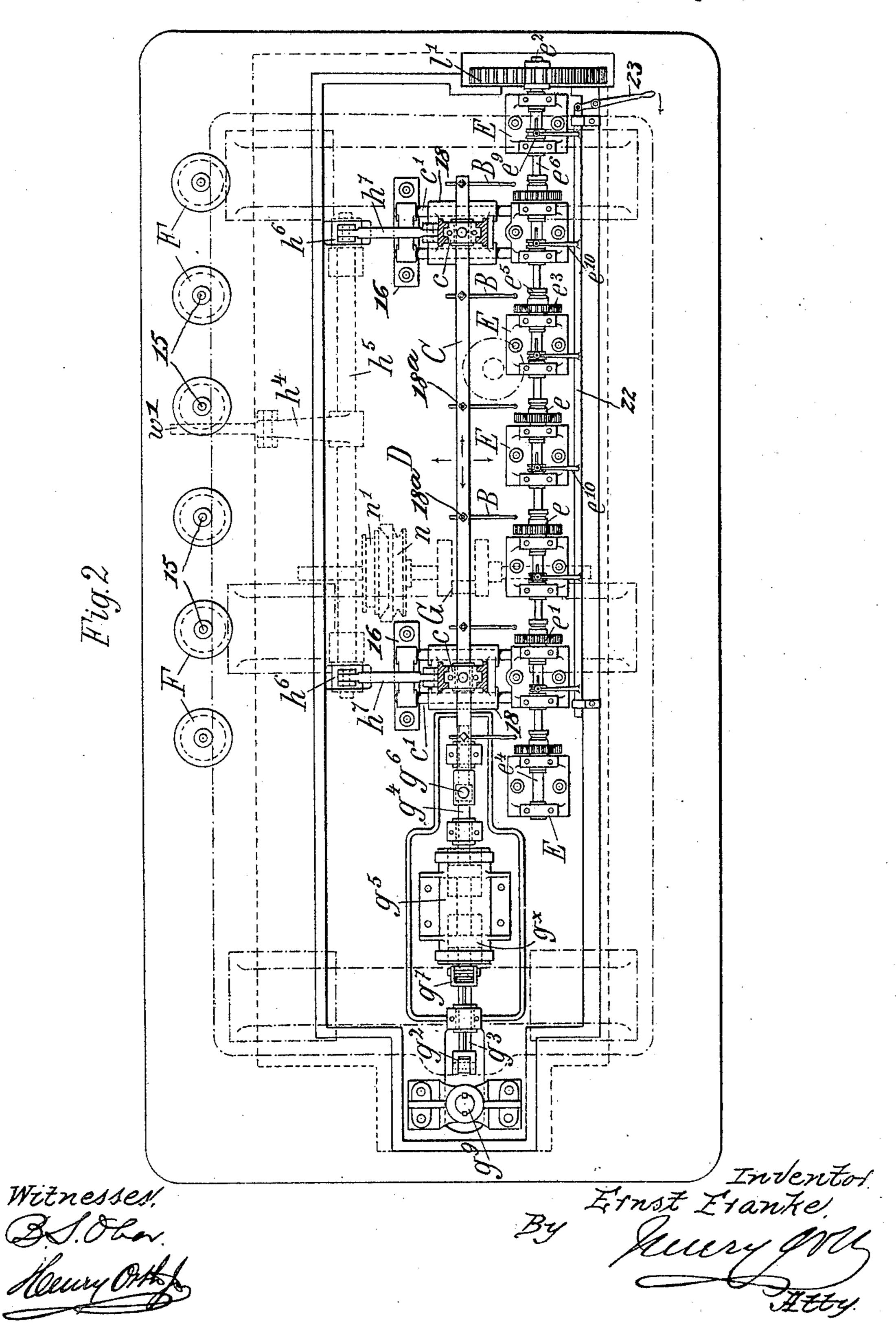
MACHINE FOR WINDING THREAD ONTO BOBBINS.
