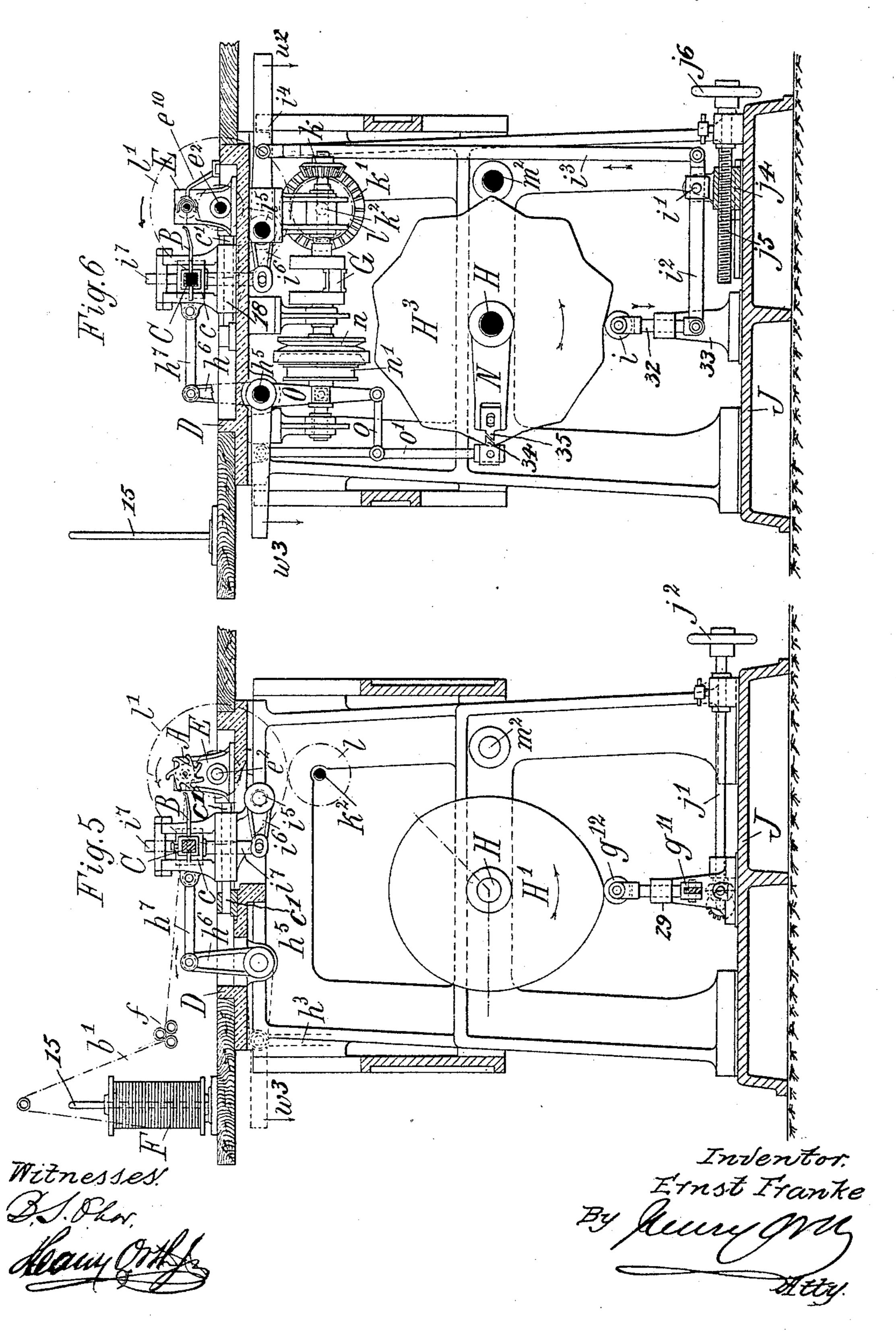
MACHINE FOR WINDING THREAD ONTO BOBBINS.
