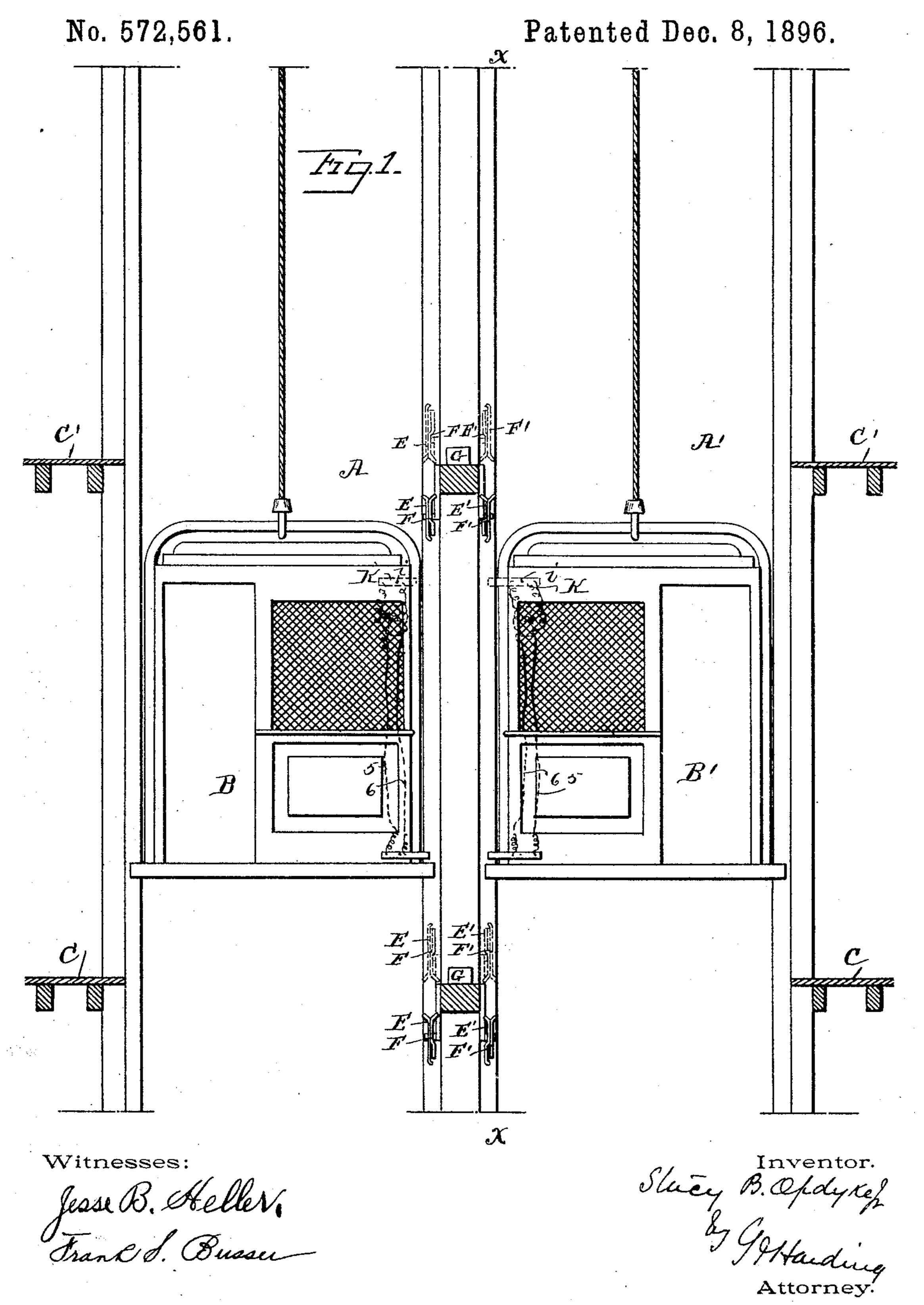
S. B. OPDYKE, Jr. ELEVATOR SIGNAL APPARATUS.
