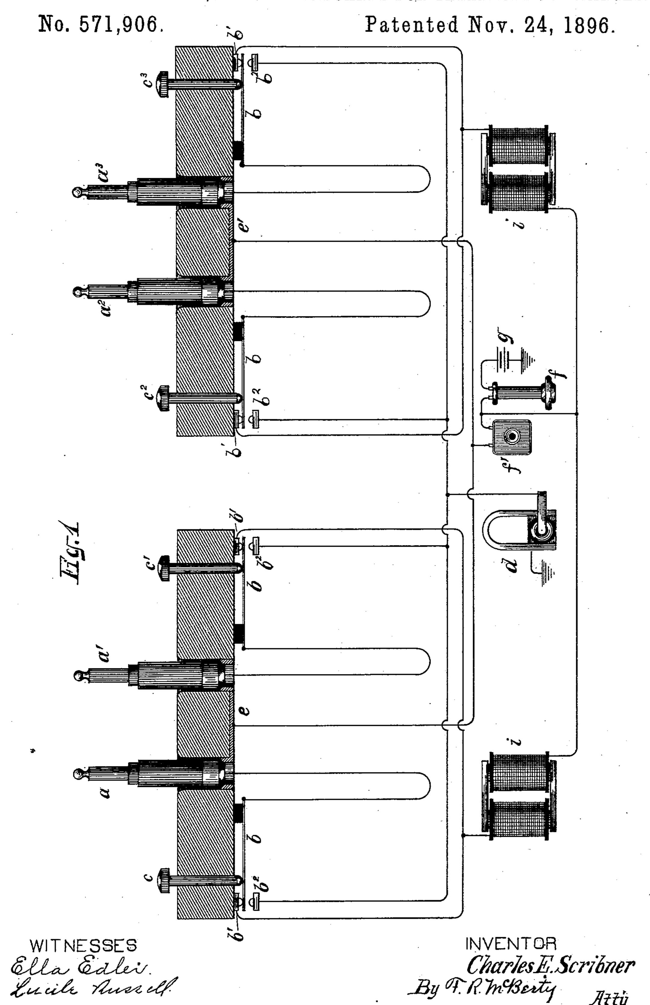
APPARATUS FOR MULTIPLE SWITCHBOARDS FOR TELEPHONE EXCHANGES.
