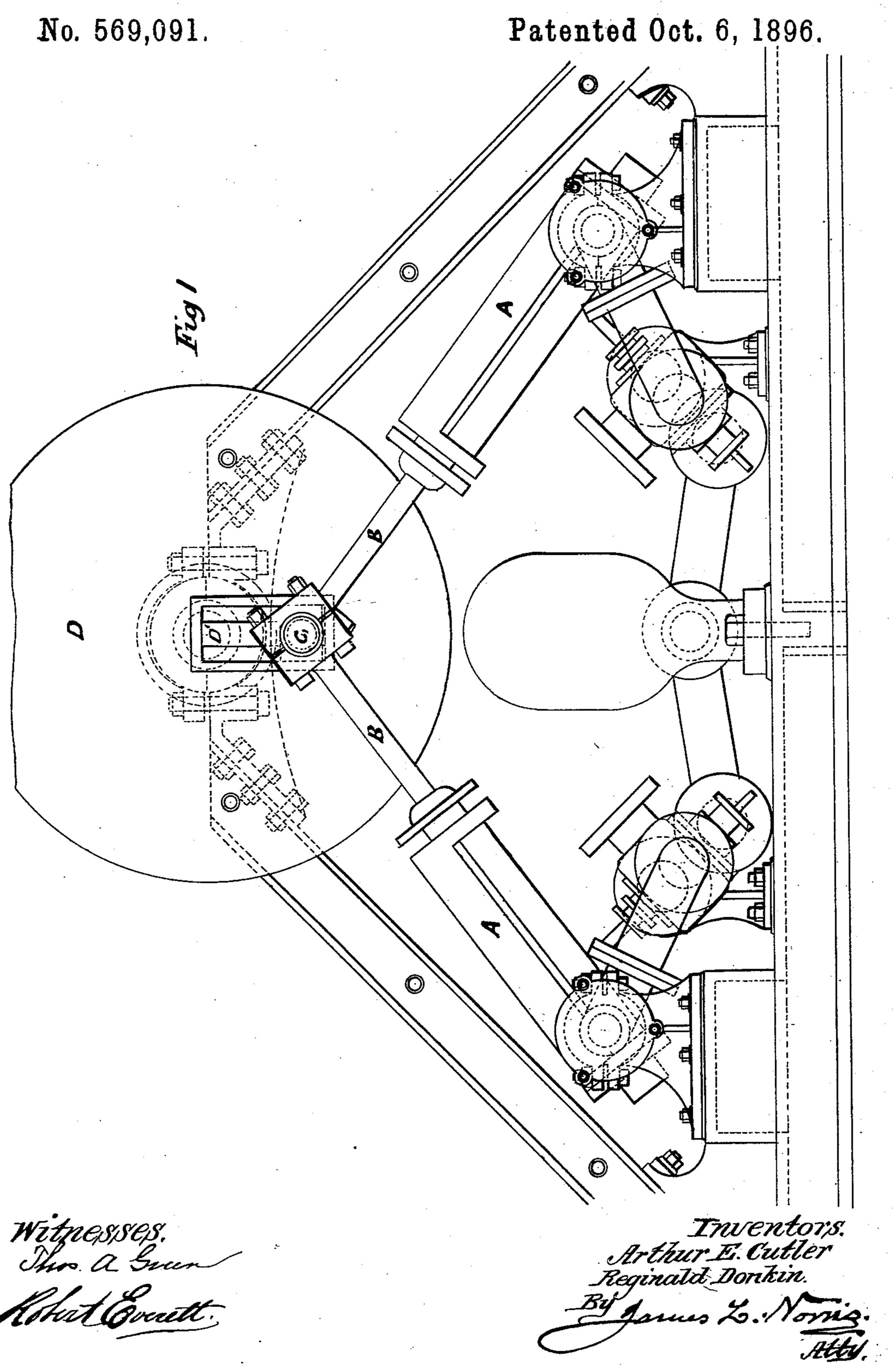
HYDRAULIC COMPENSATING PUMP OR ENGINE.
