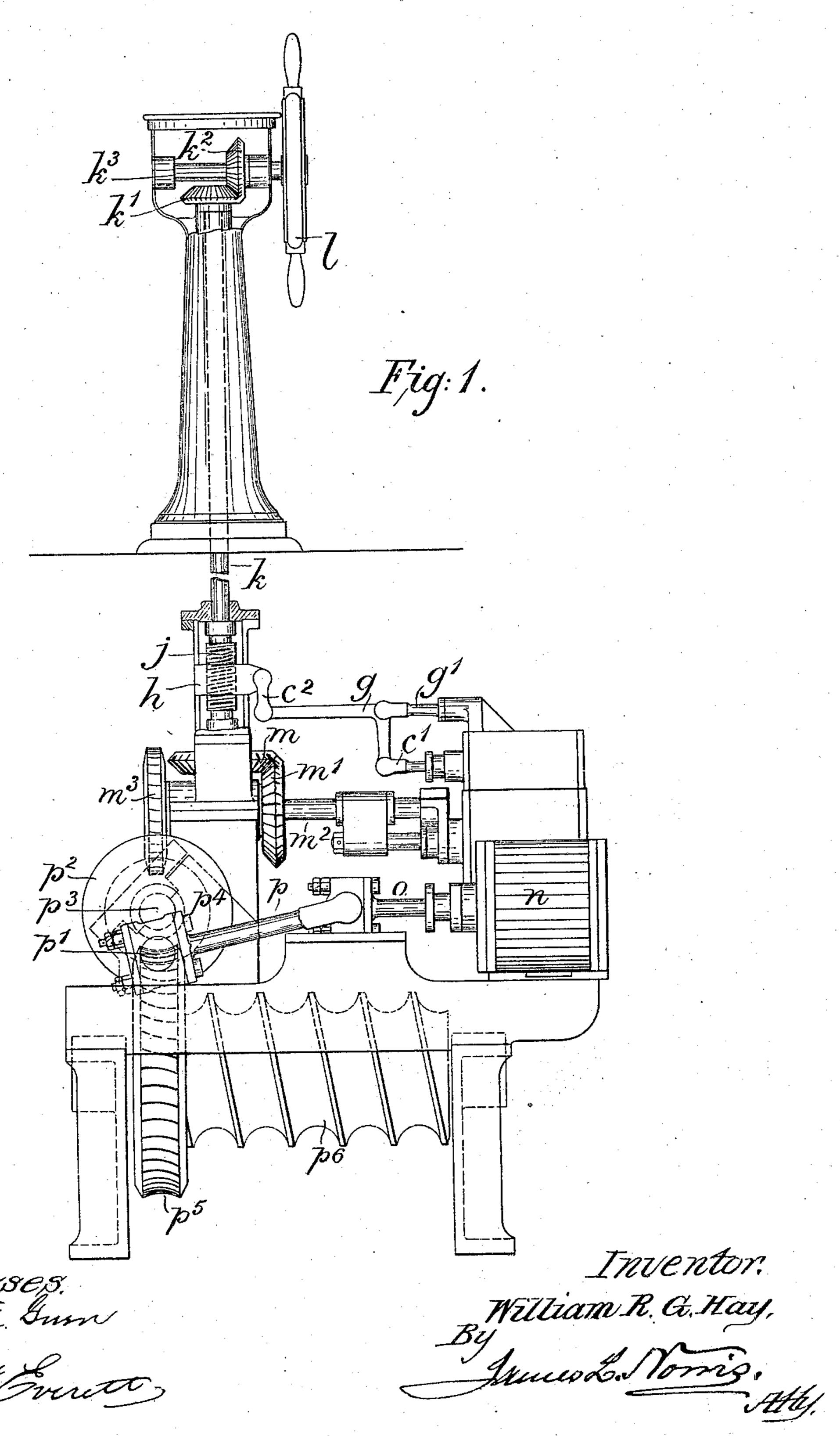
CONTROLLING VALVE APPARATUS FOR STEERING GEAR.
