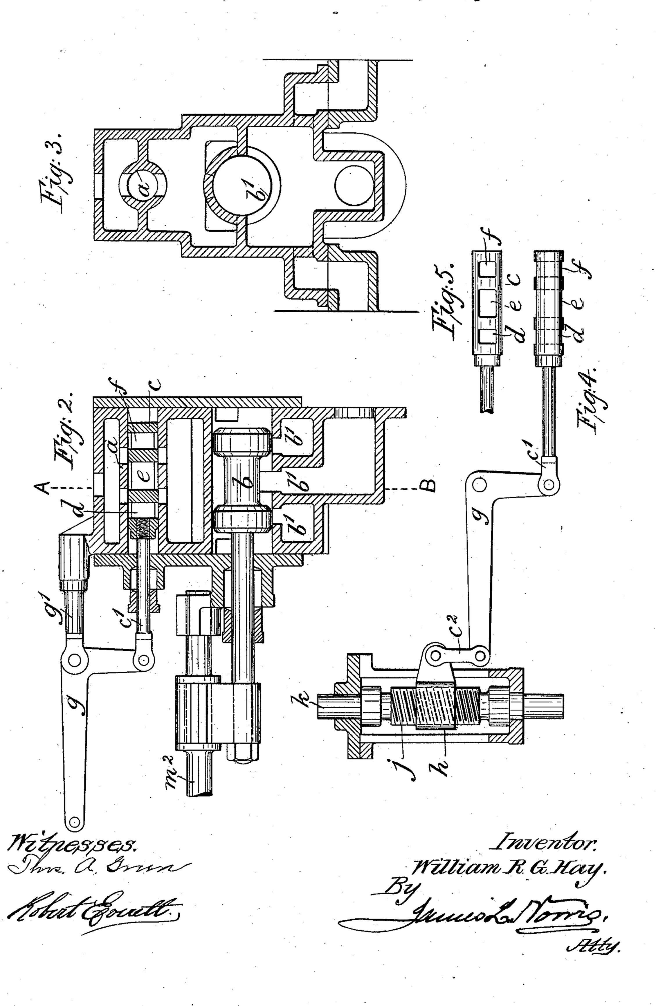
CONTROLLING VALVE APPARATUS FOR STEERING GEAR.
