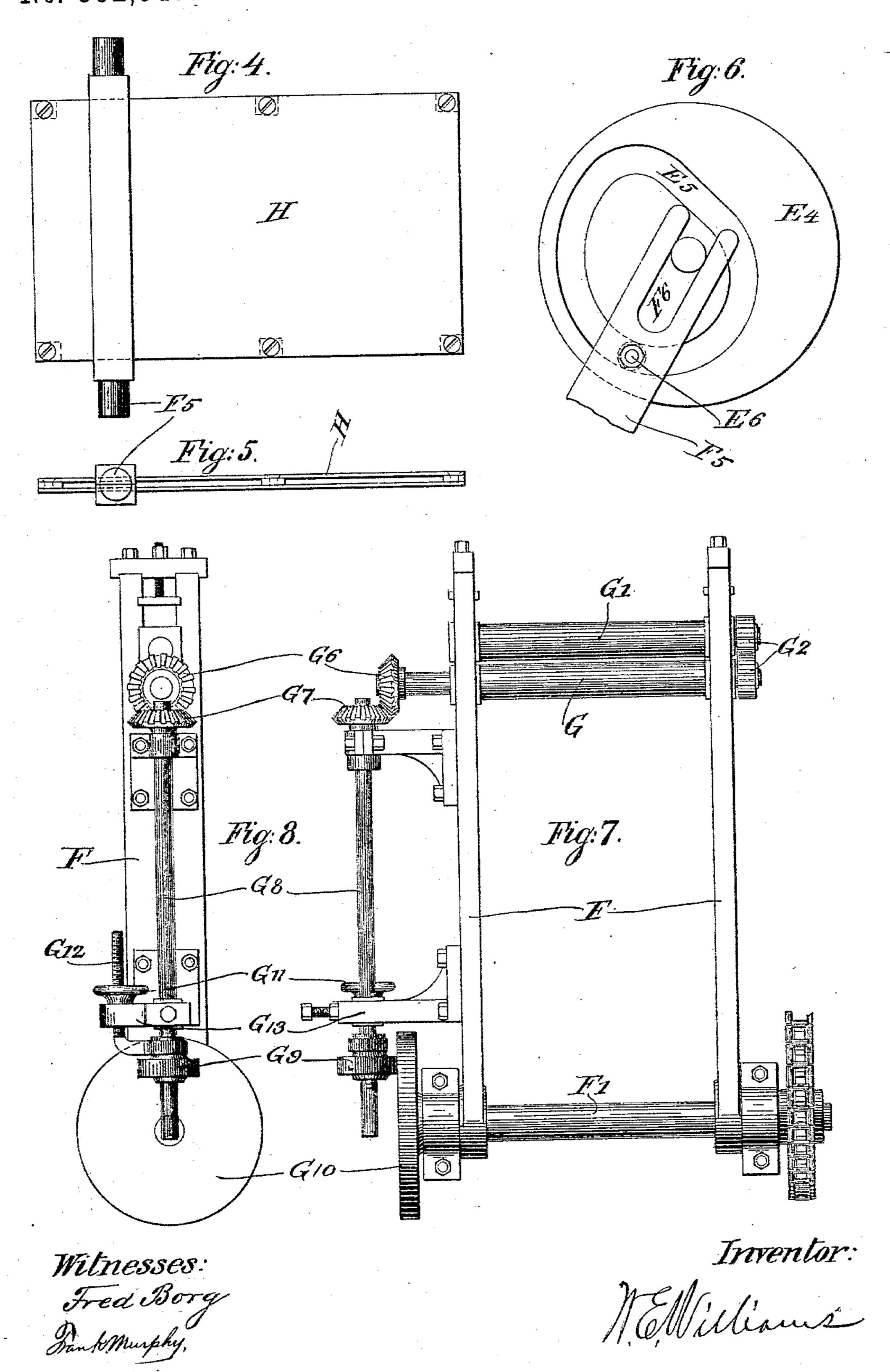
FEEDING MECHANISM FOR PAPER BOX AND PRINTING PRESS MACHINERY. No. 552,947. Patented Jan. 14, 1896.
