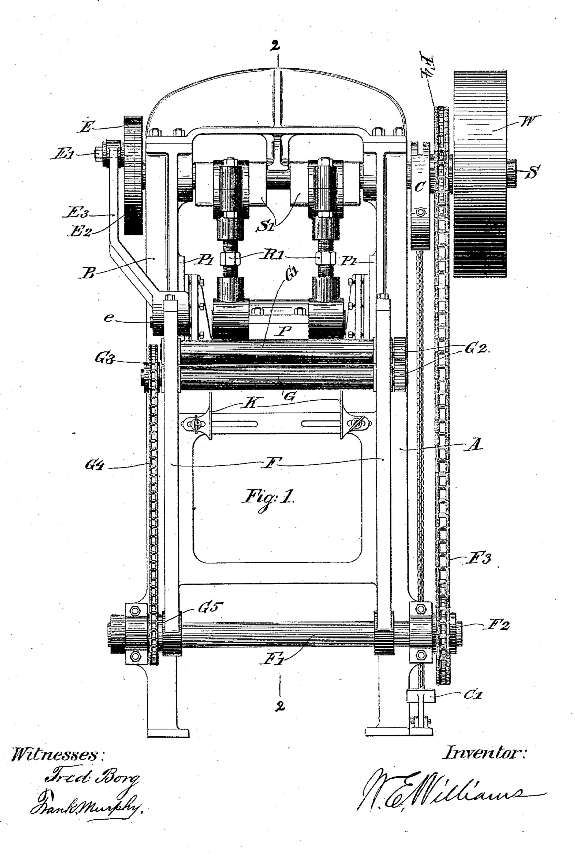
FEEDING MECHANISM FOR PAPER BOX AND PRINTING PRESS MACHINERY.
