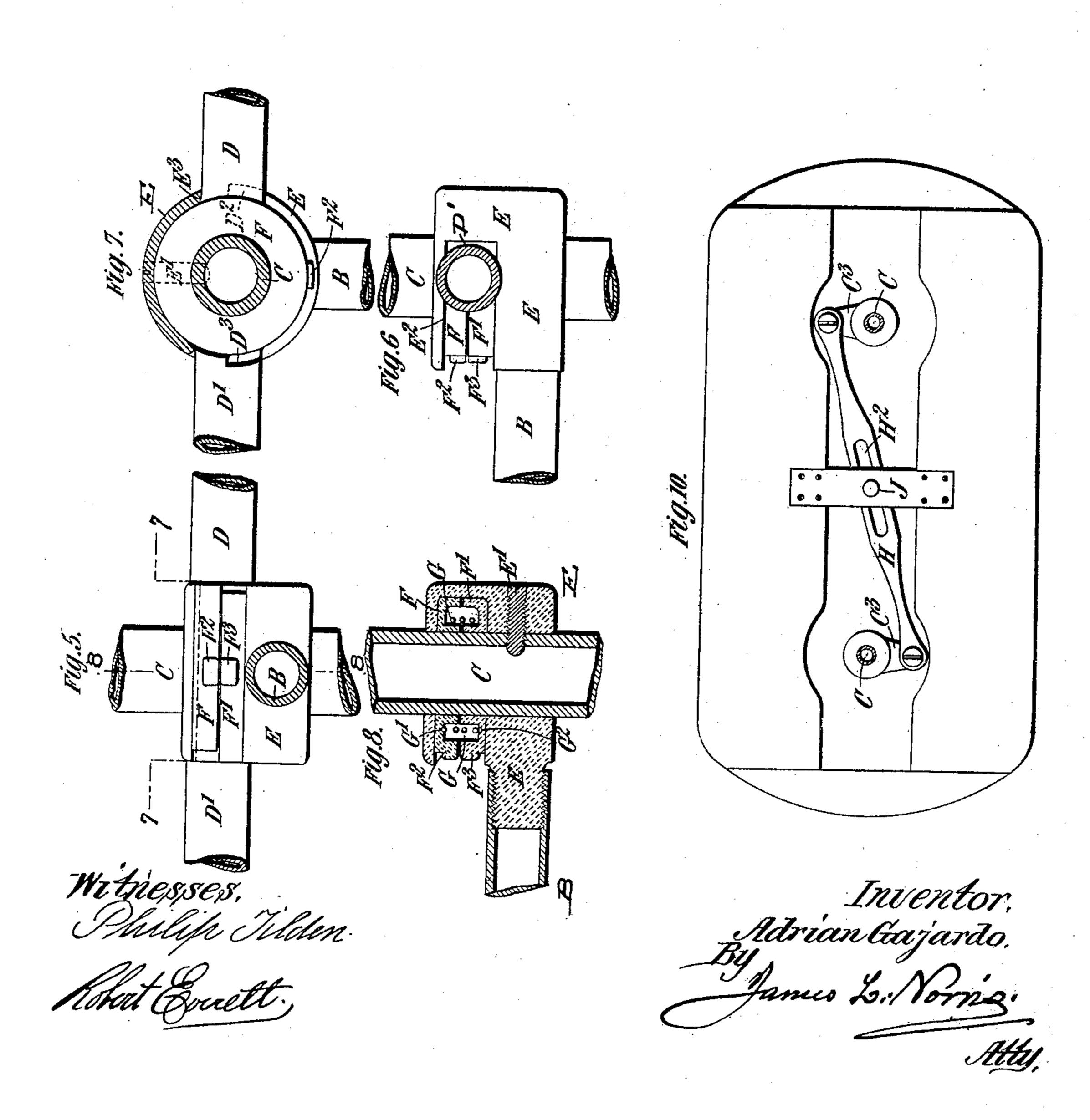
APPARATUS FOR REGISTERING THE NUMBER OF PERSONS PASSING THROUGH GATES.
