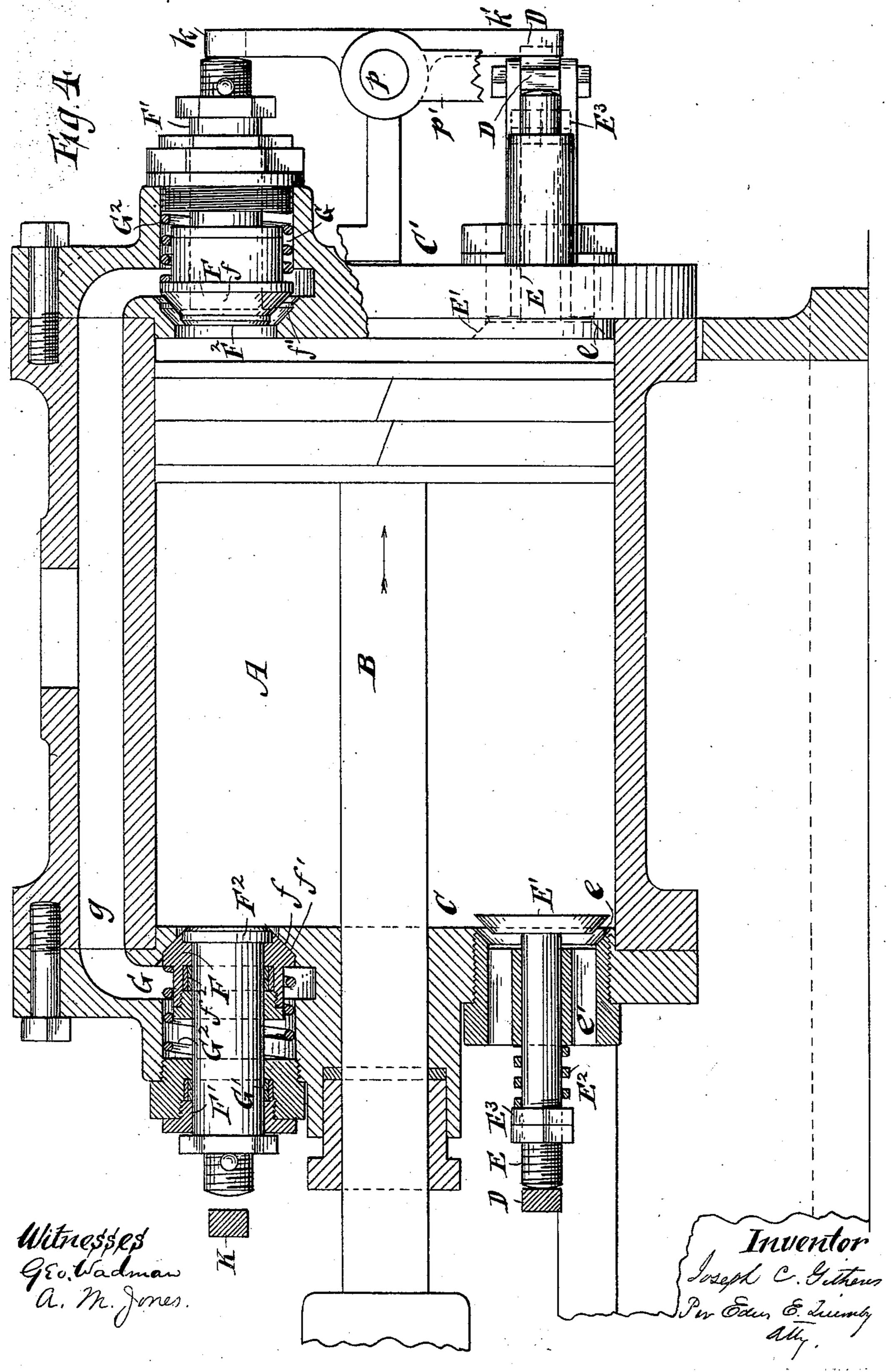
VALVE AND VALVE OPERATING MECHANISM FOR PUMPS.
