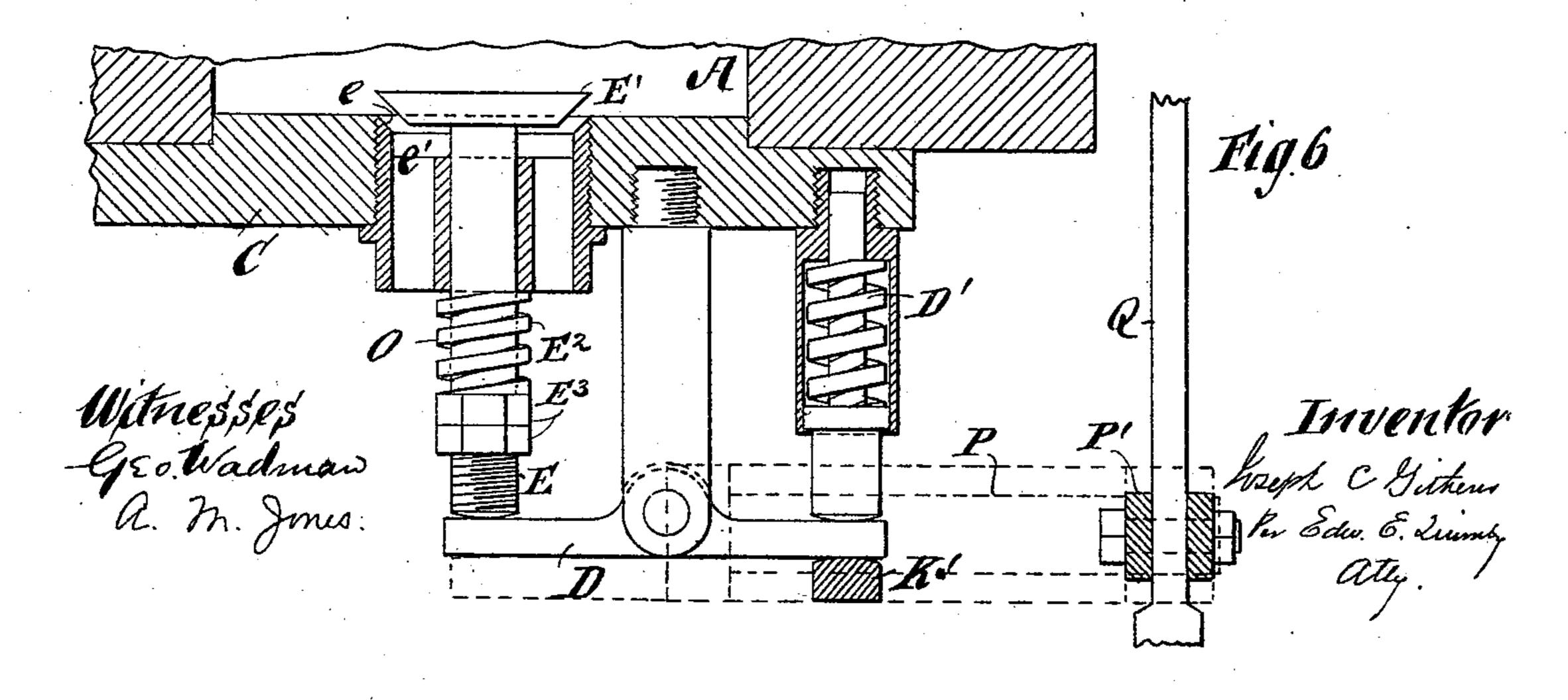
VALVE AND VALVE OPERATING MECHANISM FOR PUMPS.
