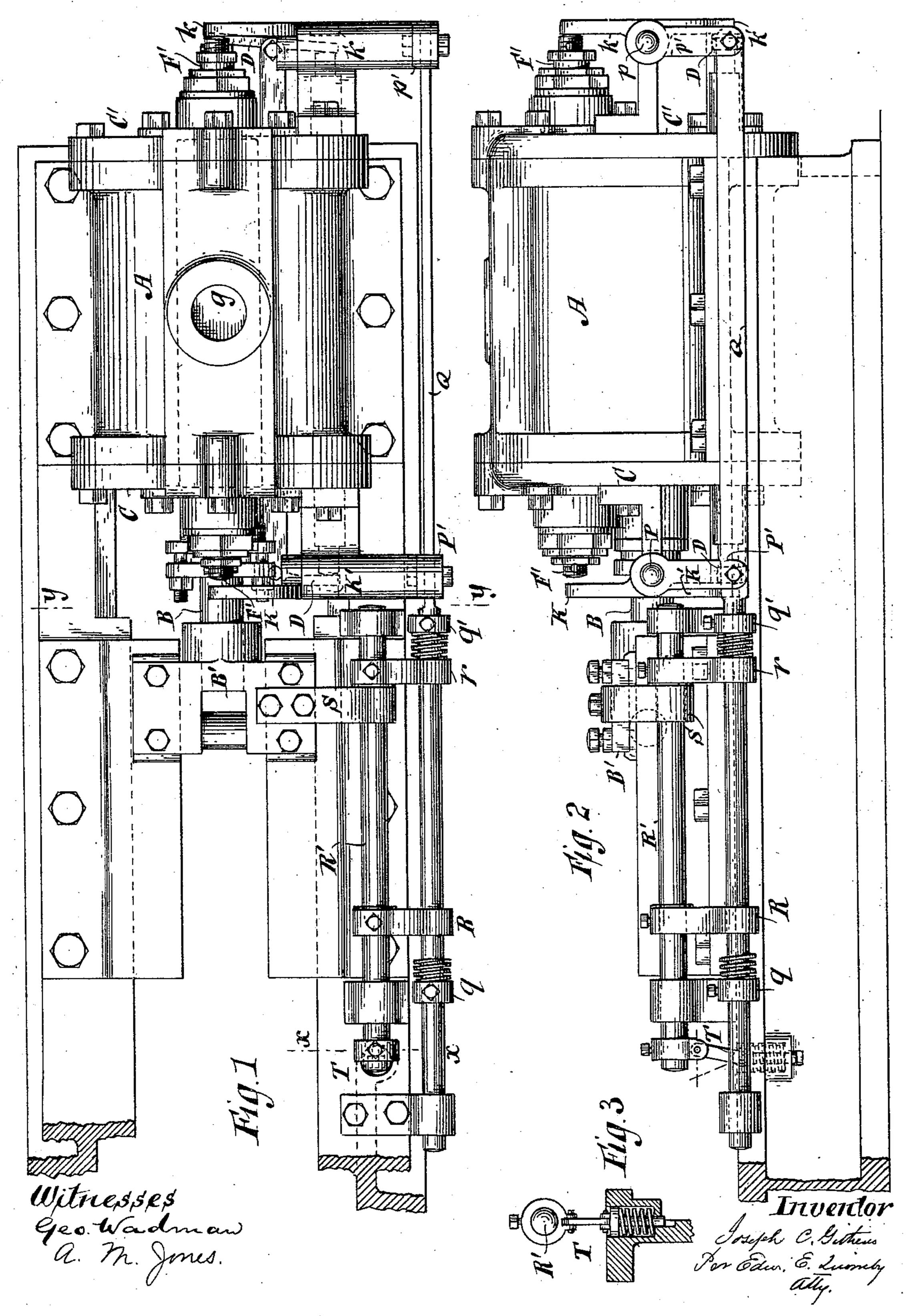
VALVE AND VALVE OPERATING MECHANISM FOR PUMPS.
