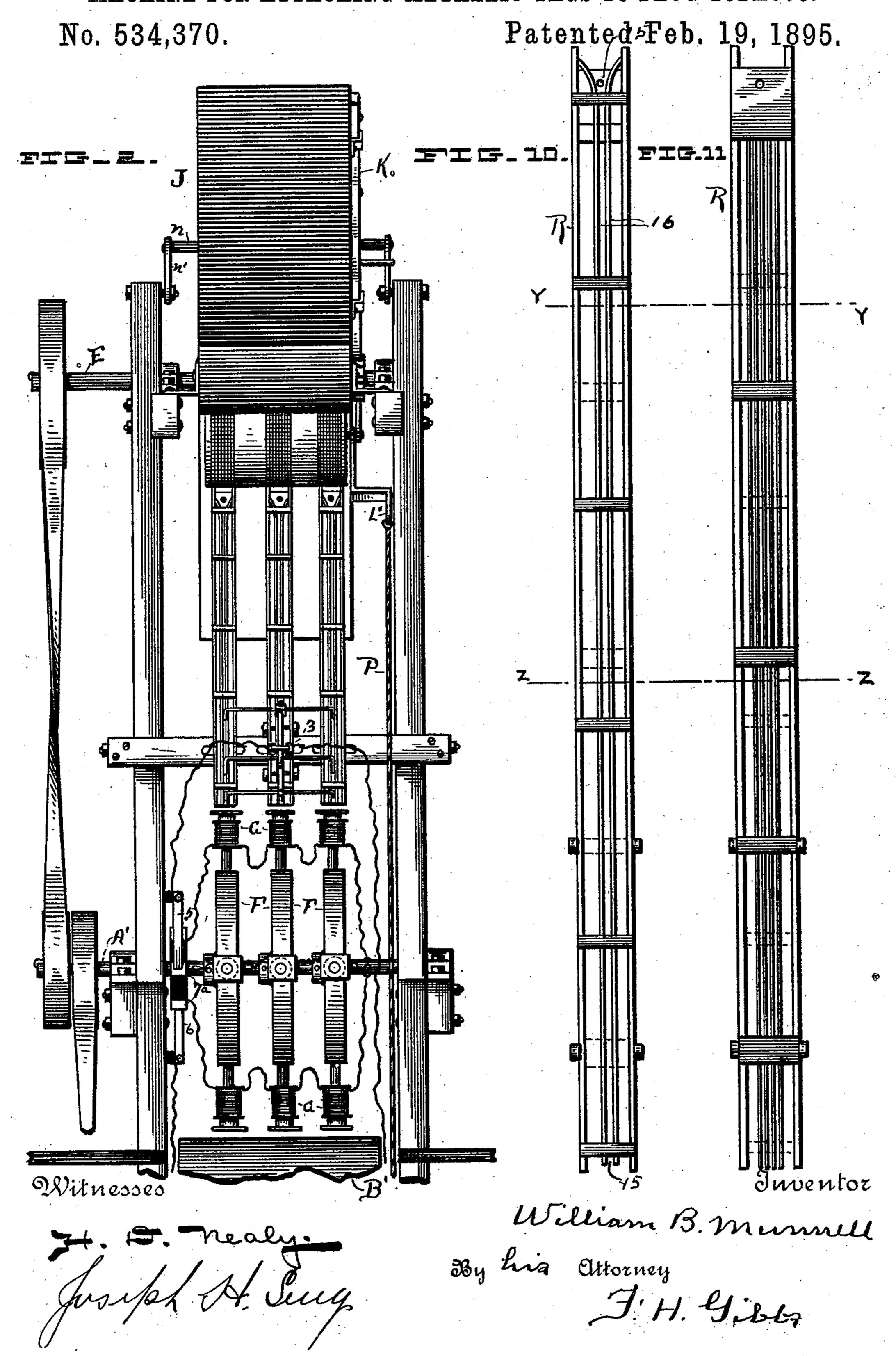
MACHINE FOR ATTACHING METALLIC TAGS TO PLUG TOBACCO.
