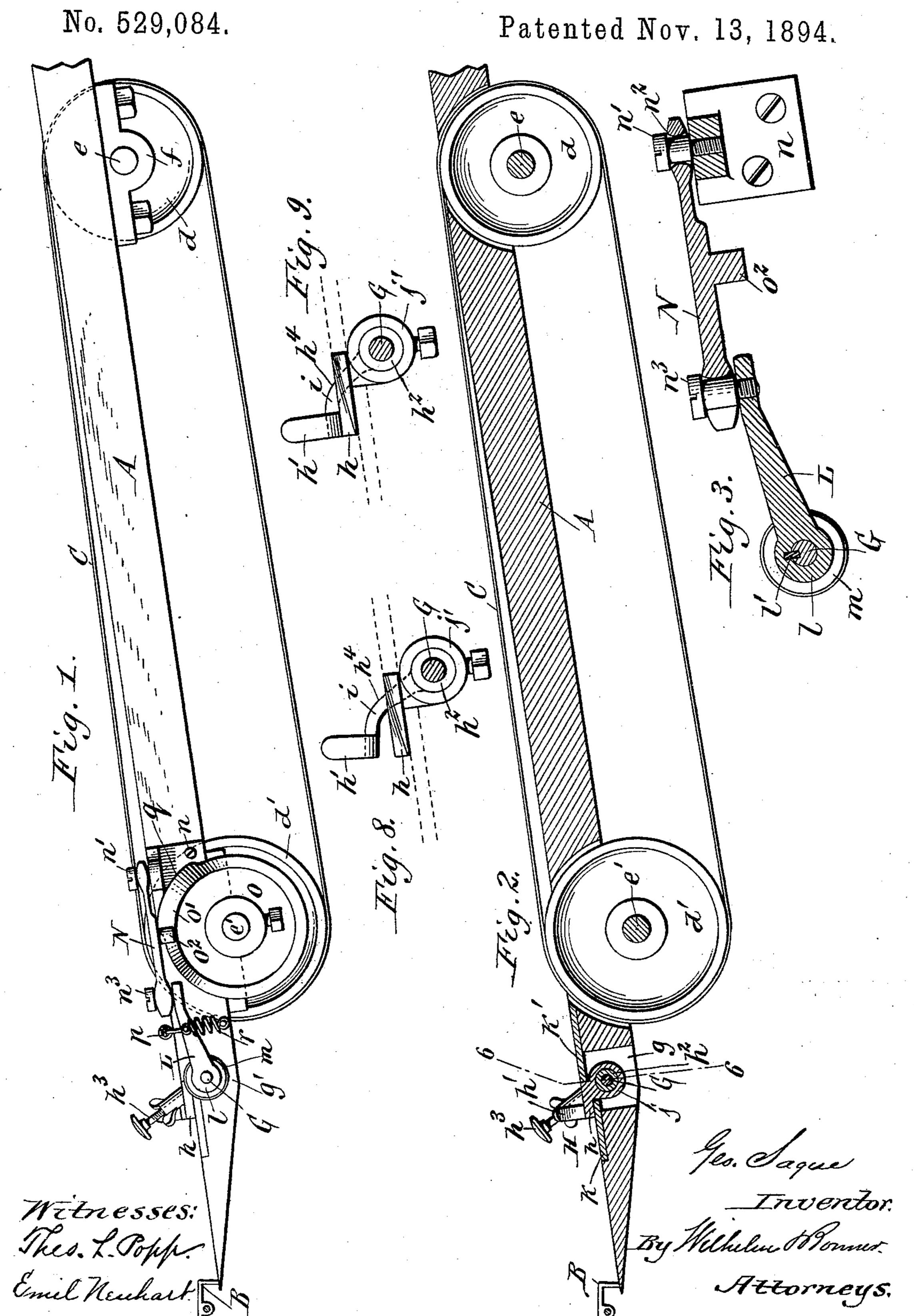
SIDE REGISTERING MECHANISM FOR PAPER FEEDERS.
