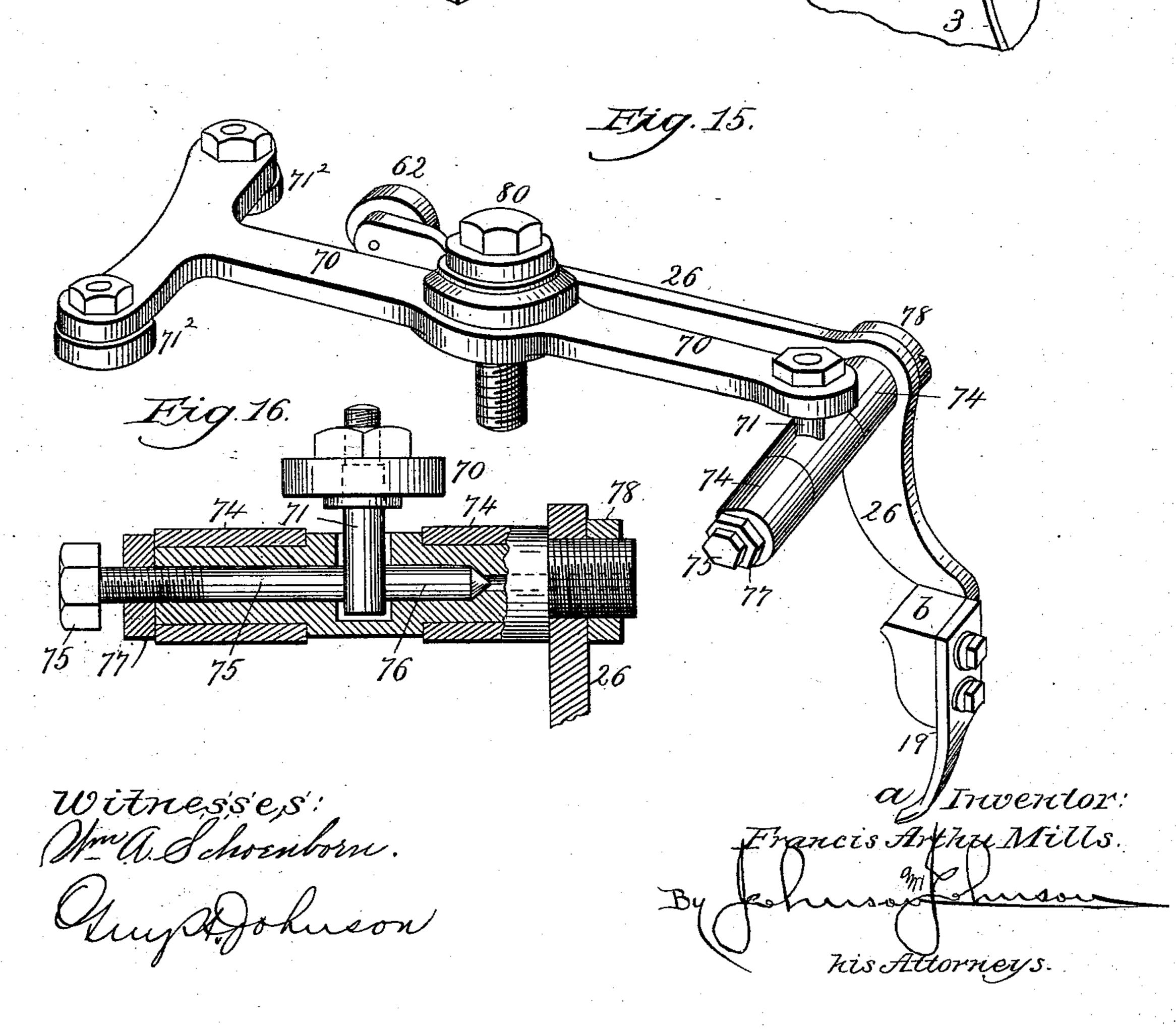
WORK SUPPORTING AND FEEDING DEVICE FOR SHOE SEWING MACHINES.
