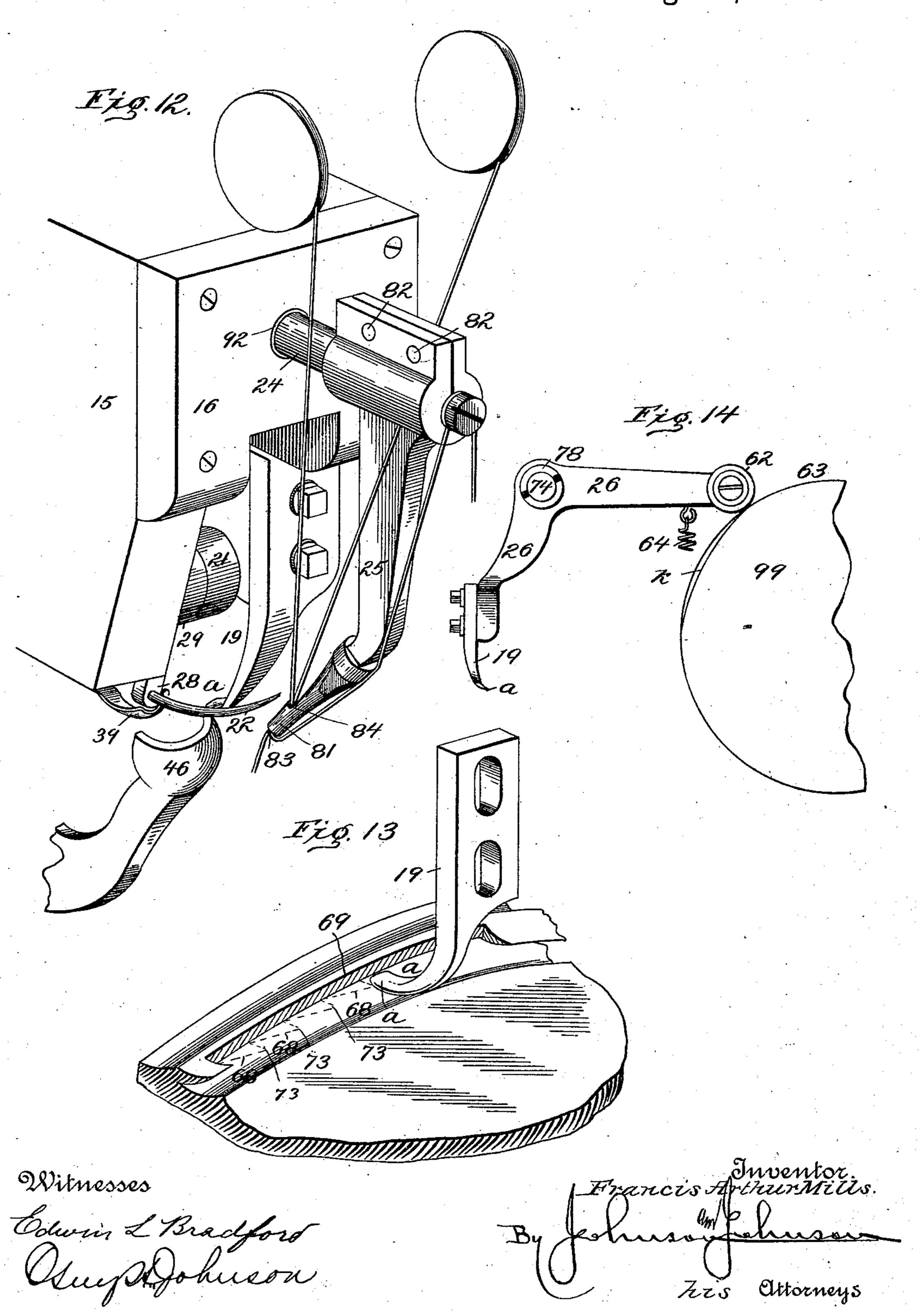
WORK SUPPORTING AND FEEDING DEVICE FOR SHOE SEWING MACHINES. Patented Aug. 14, 1894.
