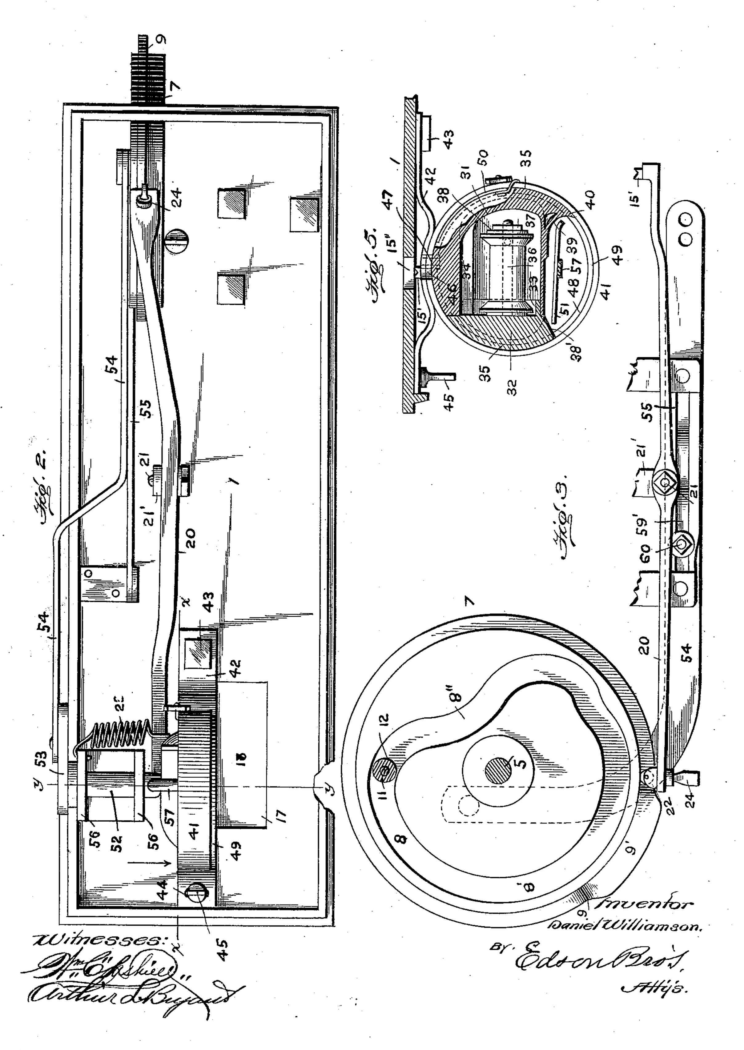
SHUTTLE AND SHUTTLE ACTUATING MECHANISM FOR SEWING MACHINES.
