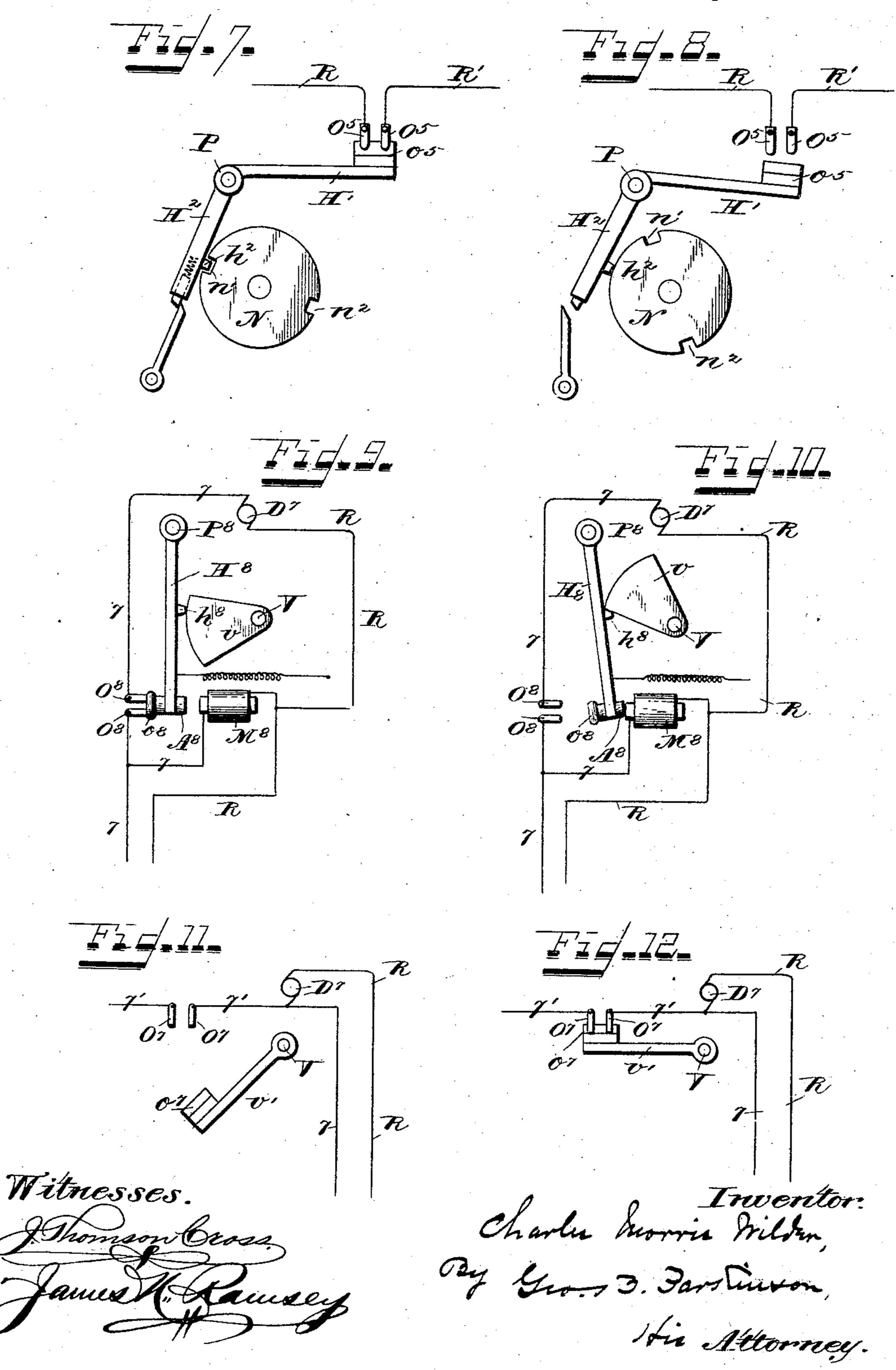
ELECTRIC CONTROLLING AND LOCKING MECHANISM FOR RAILWAY SWITCHES AND SIGNALS
