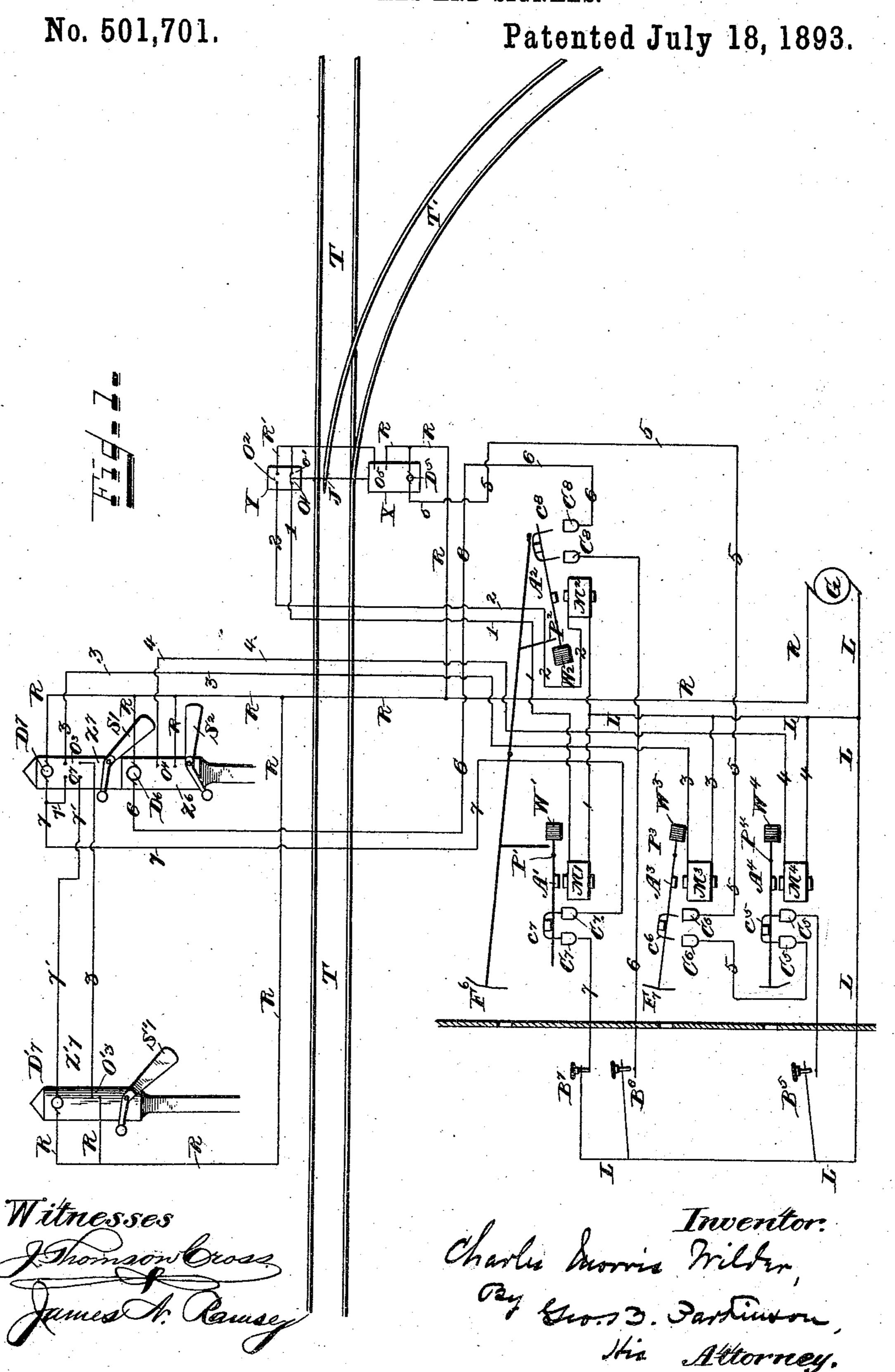
ELECTRIC CONTROLLING AND LOCKING MECHANISM FOR RAILWAY SWITCHES AND SIGNALS.
