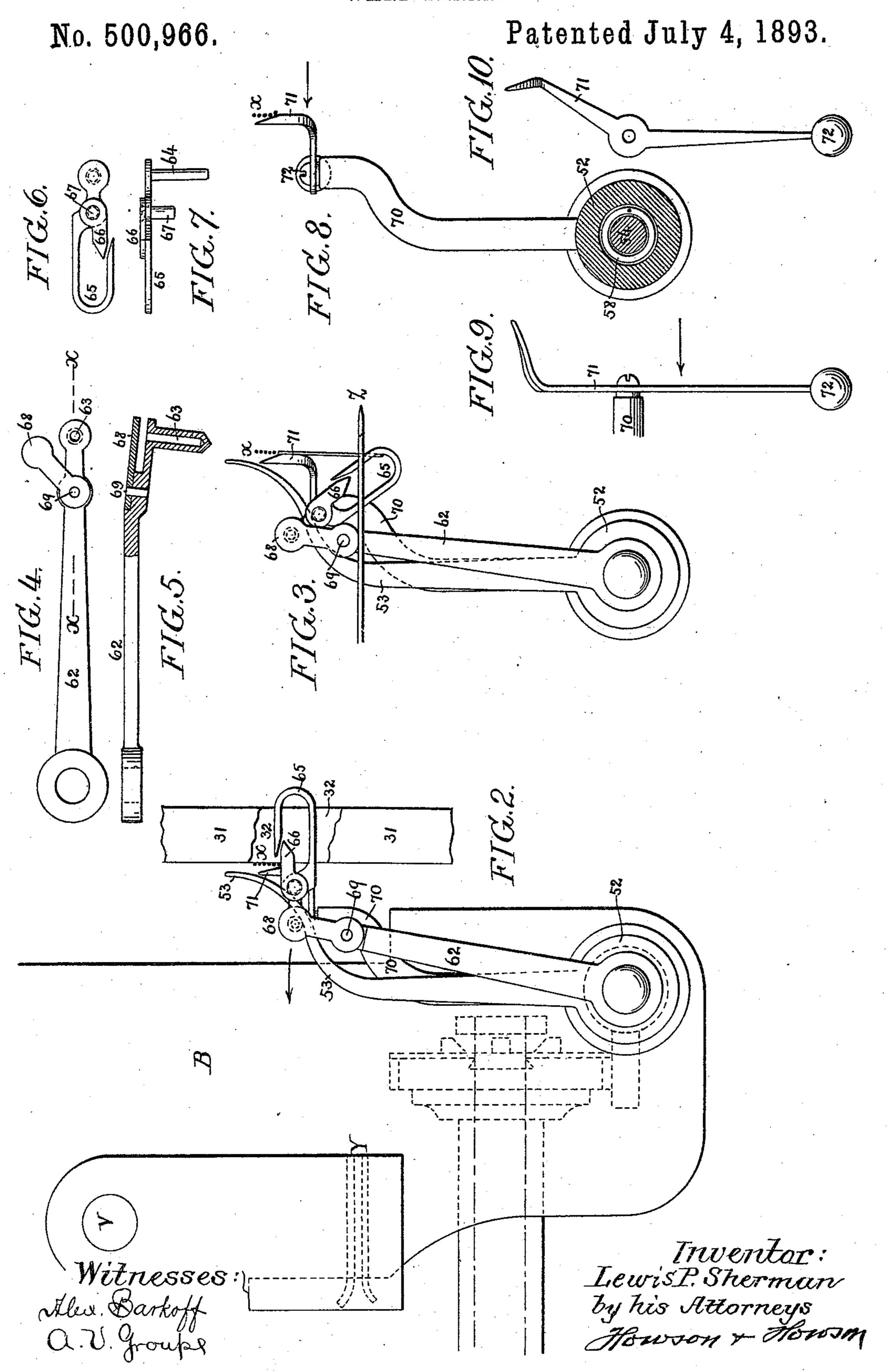
THREAD SELECTING DEVICE FOR MACHINES FOR DRAWING IN WARP THREADS.
