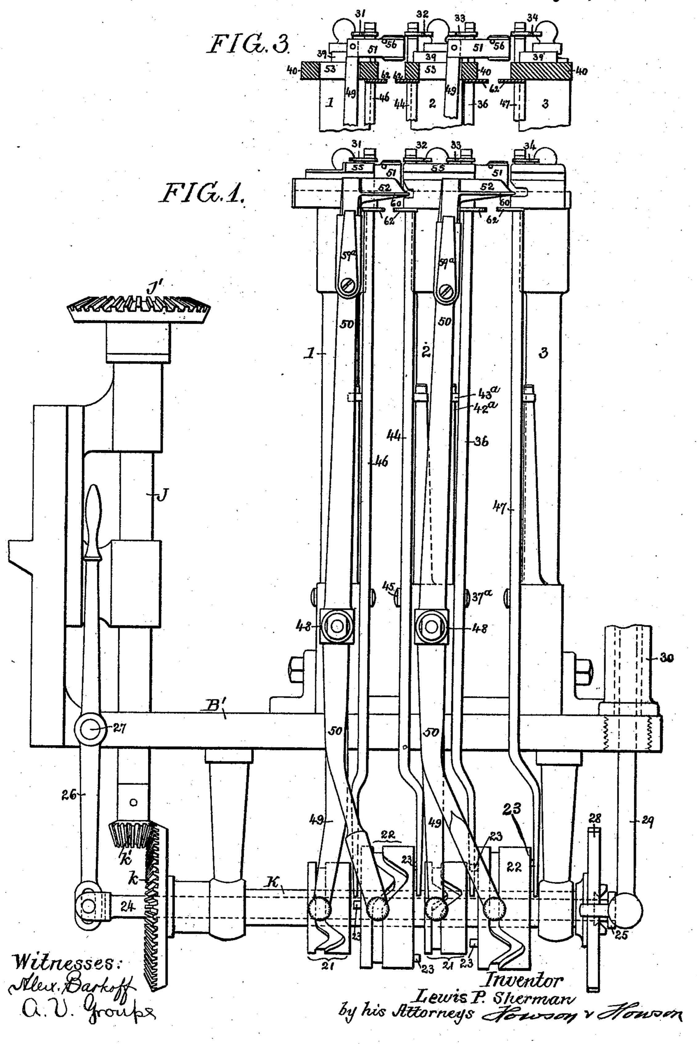
HARNESS SUPPORTING AND HEDDLE EYE SELECTING DEVICE FOR MACHINES FOR DRAWING IN WARP THREADS.
