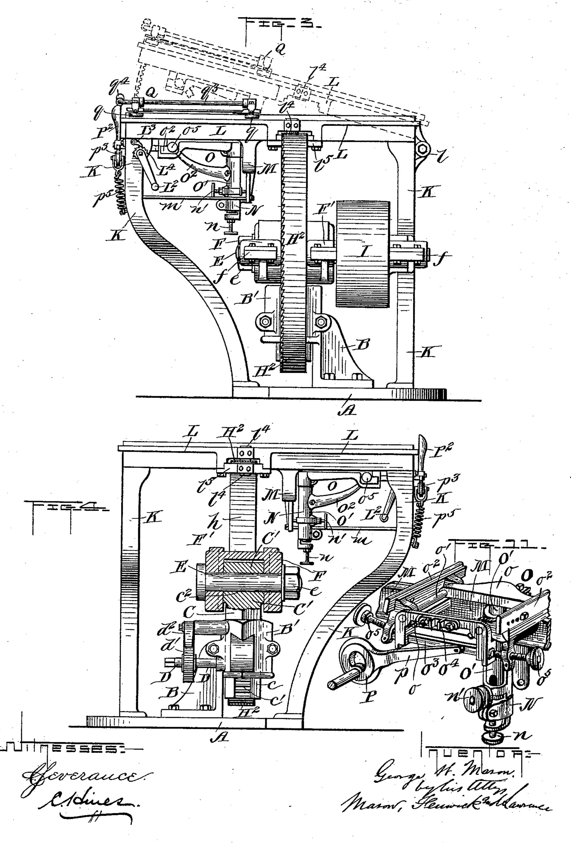
BAND SAW SHINGLE OR BOARD SAWING MACHINE.
