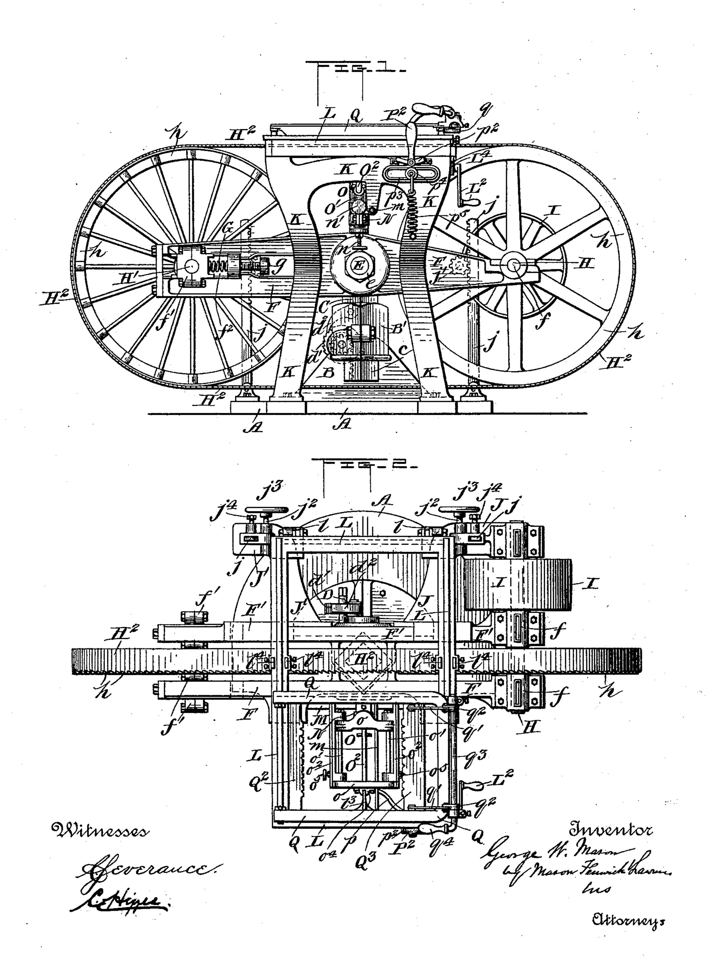
BAND SAW SHINGLE OR BOARD SAWING MACHINE.
