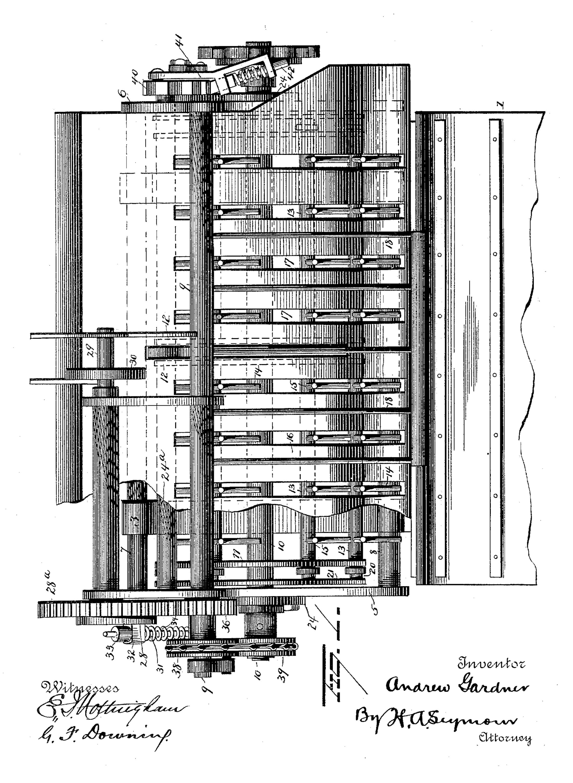
ELEVATING AND PACKING MECHANISM FOR HARVESTERS.
