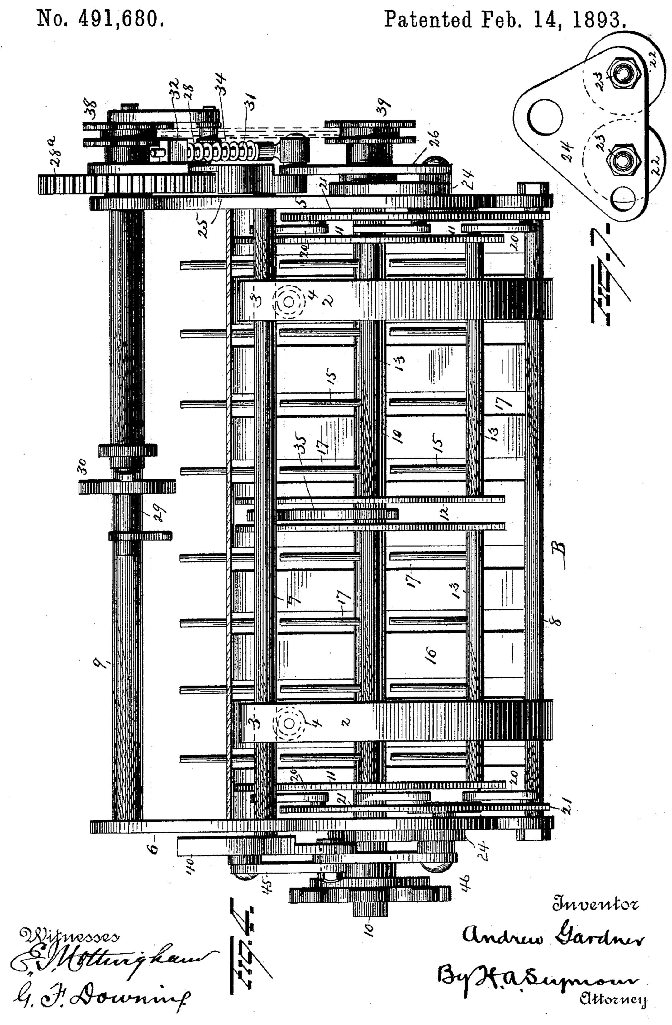
ELEVATING AND PACKING MECHANISM FOR HARVESTERS.
