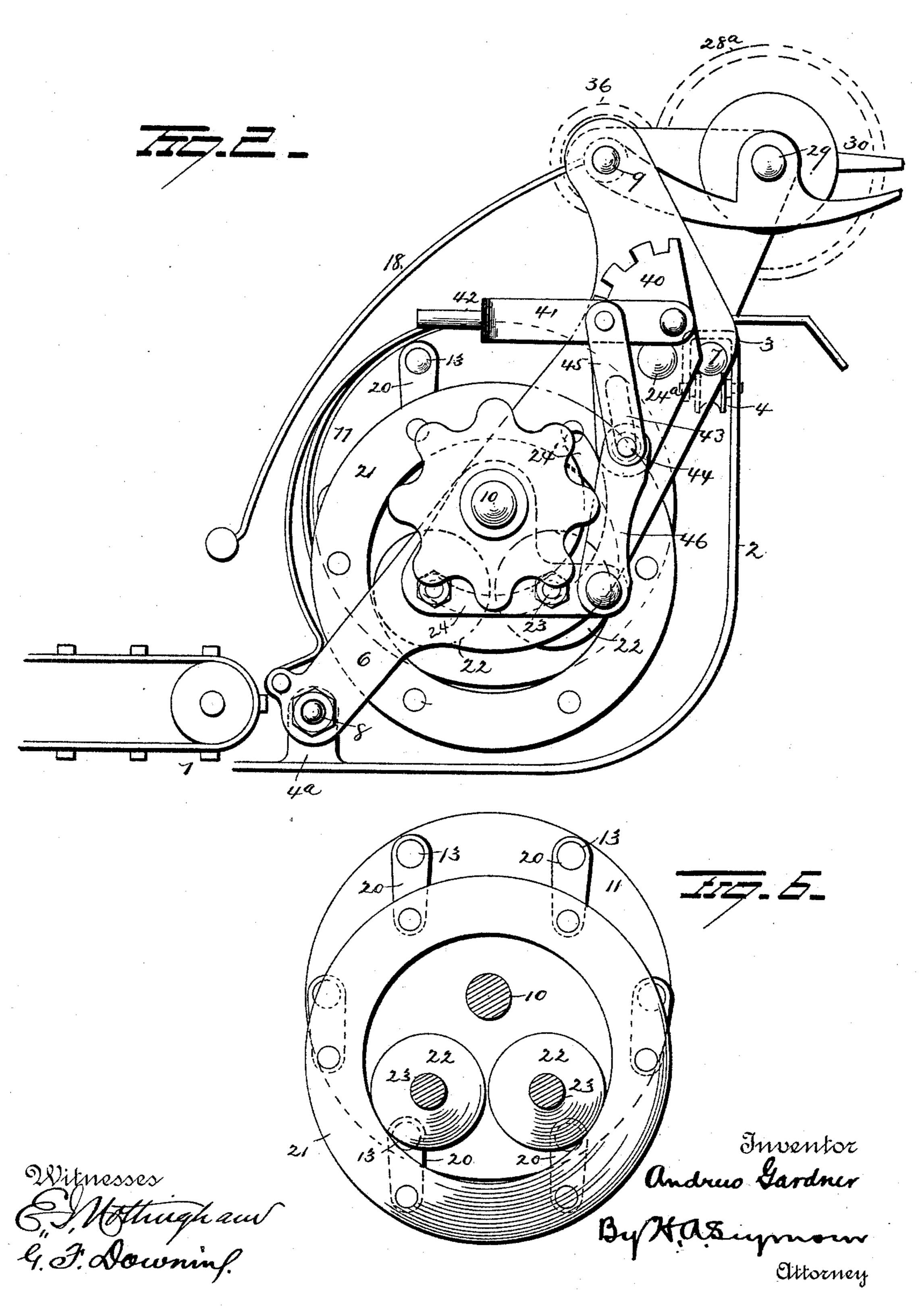
ELEVATING AND PACKING MECHANISM FOR HARVESTERS.
