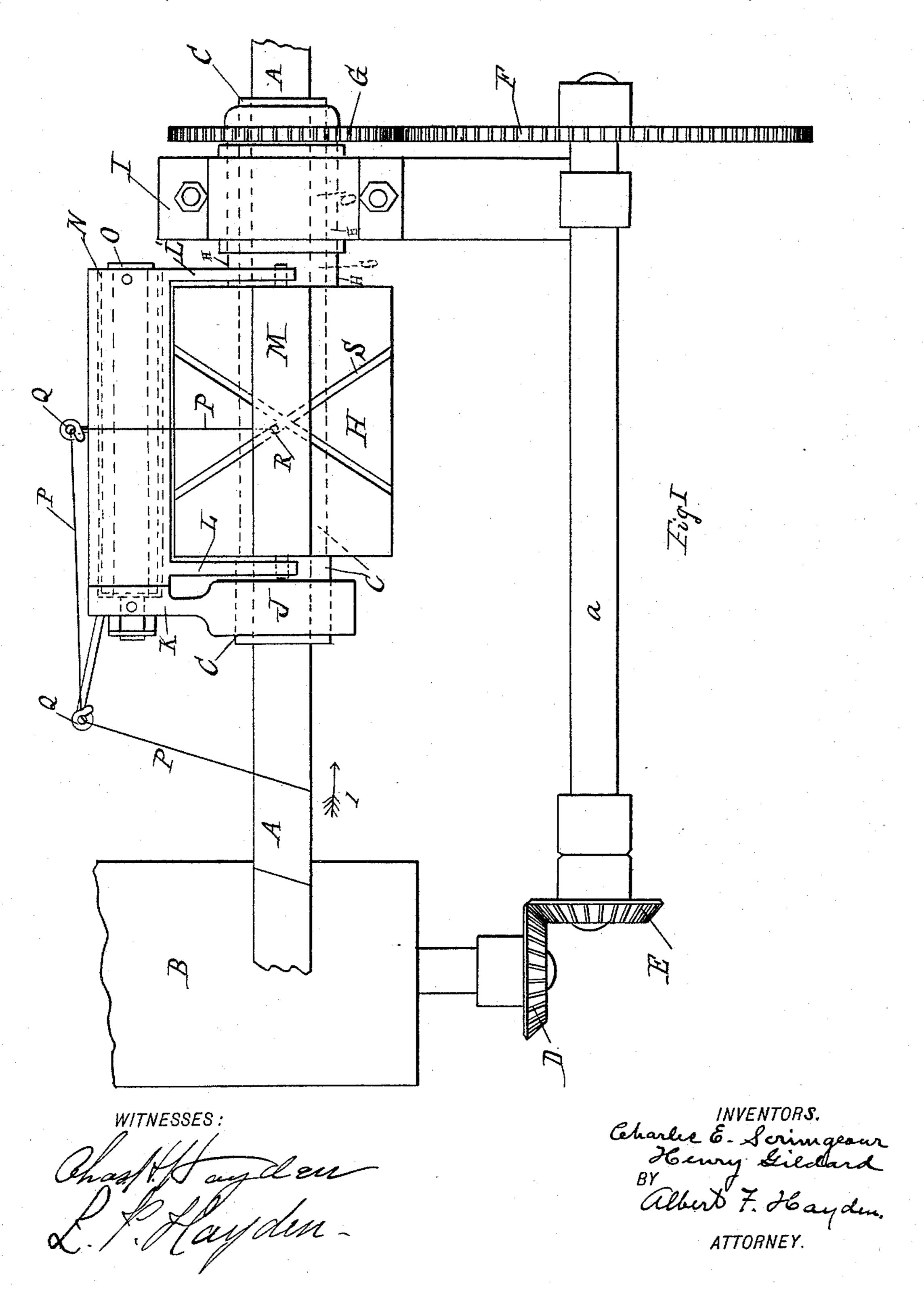
C. E. SCRIMGEOUR & H. GILDARD. MECHANISM FOR UNWINDING WARP THREADS.
