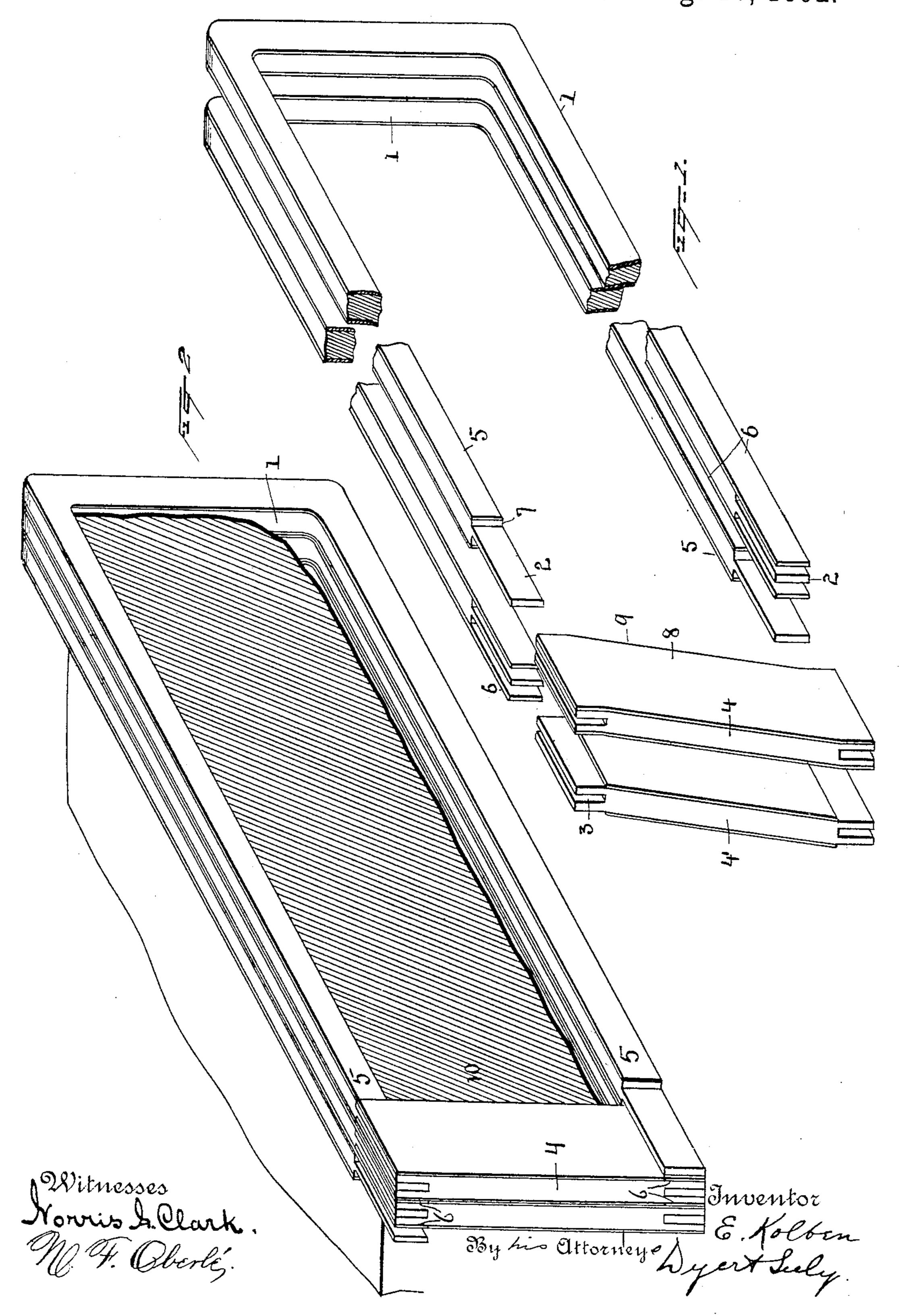
ARMATURE CONDUCTOR AND MEANS FOR INSULATING THE SAME.
