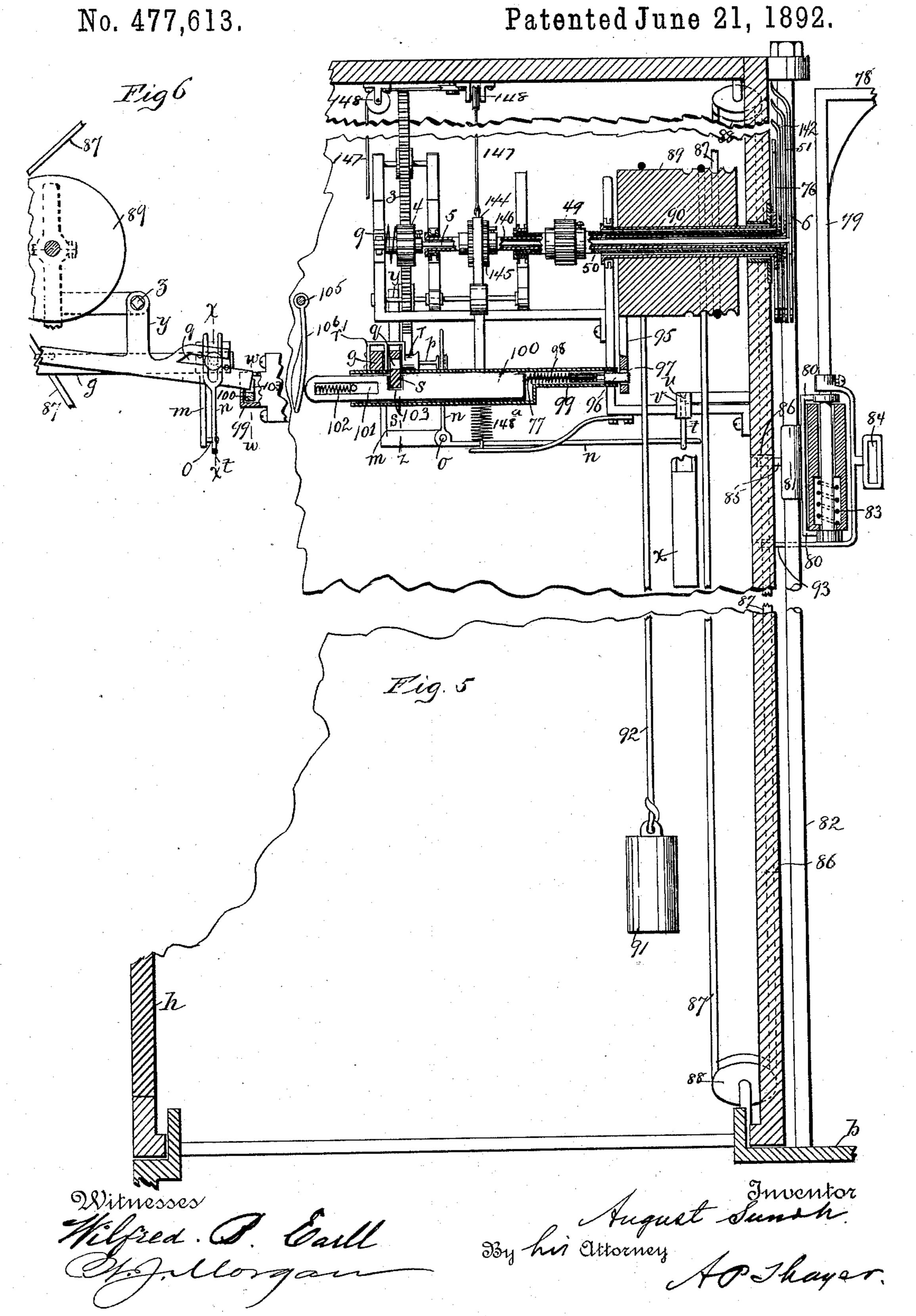
COMBINED WEIGHING, LIFTING, MEASURING, AND ELECTRIC MACHINE.
