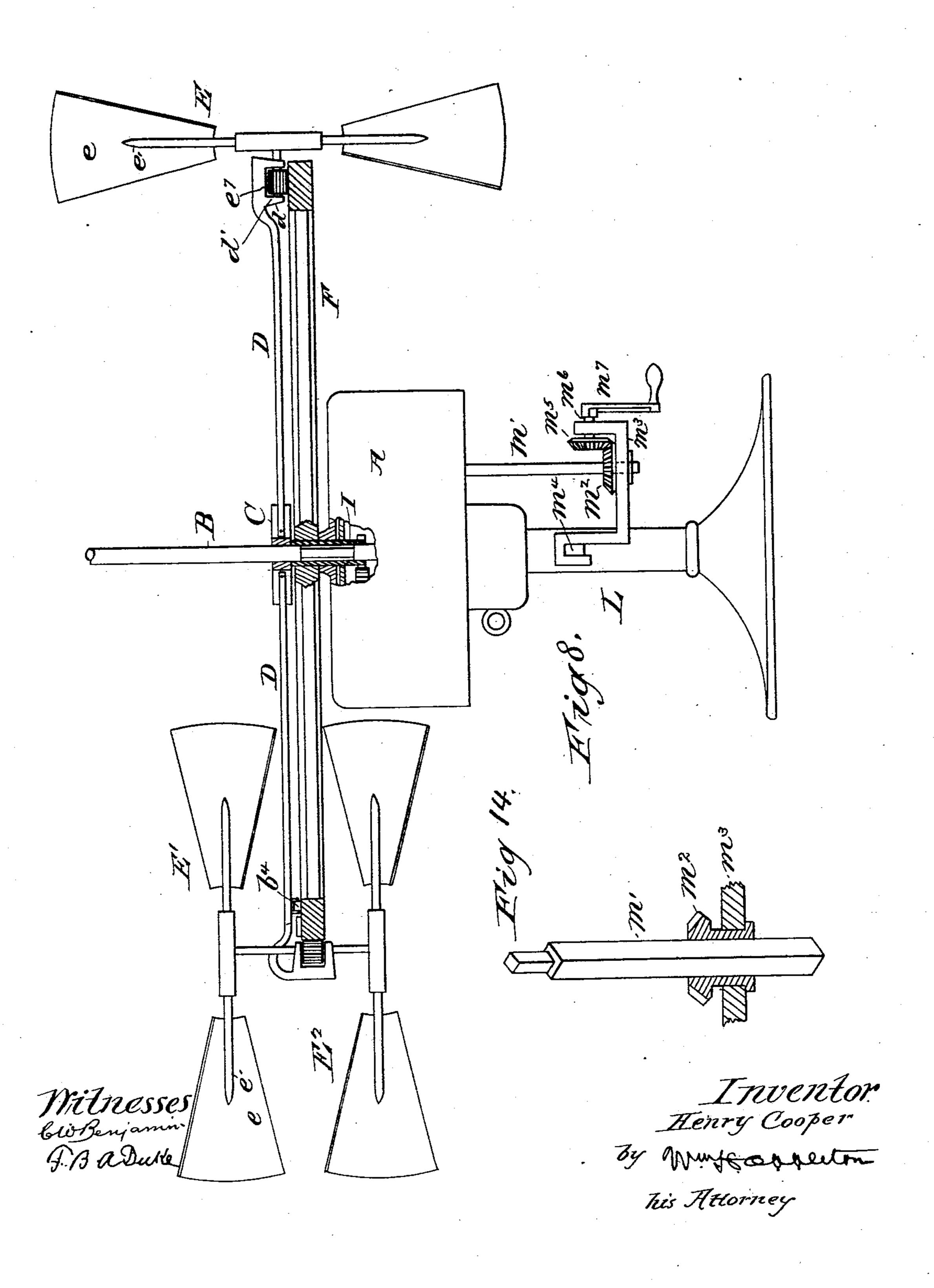
MACHINE FOR AGITATING AND CIRCULATING AIR IN ROOMS, &c.
