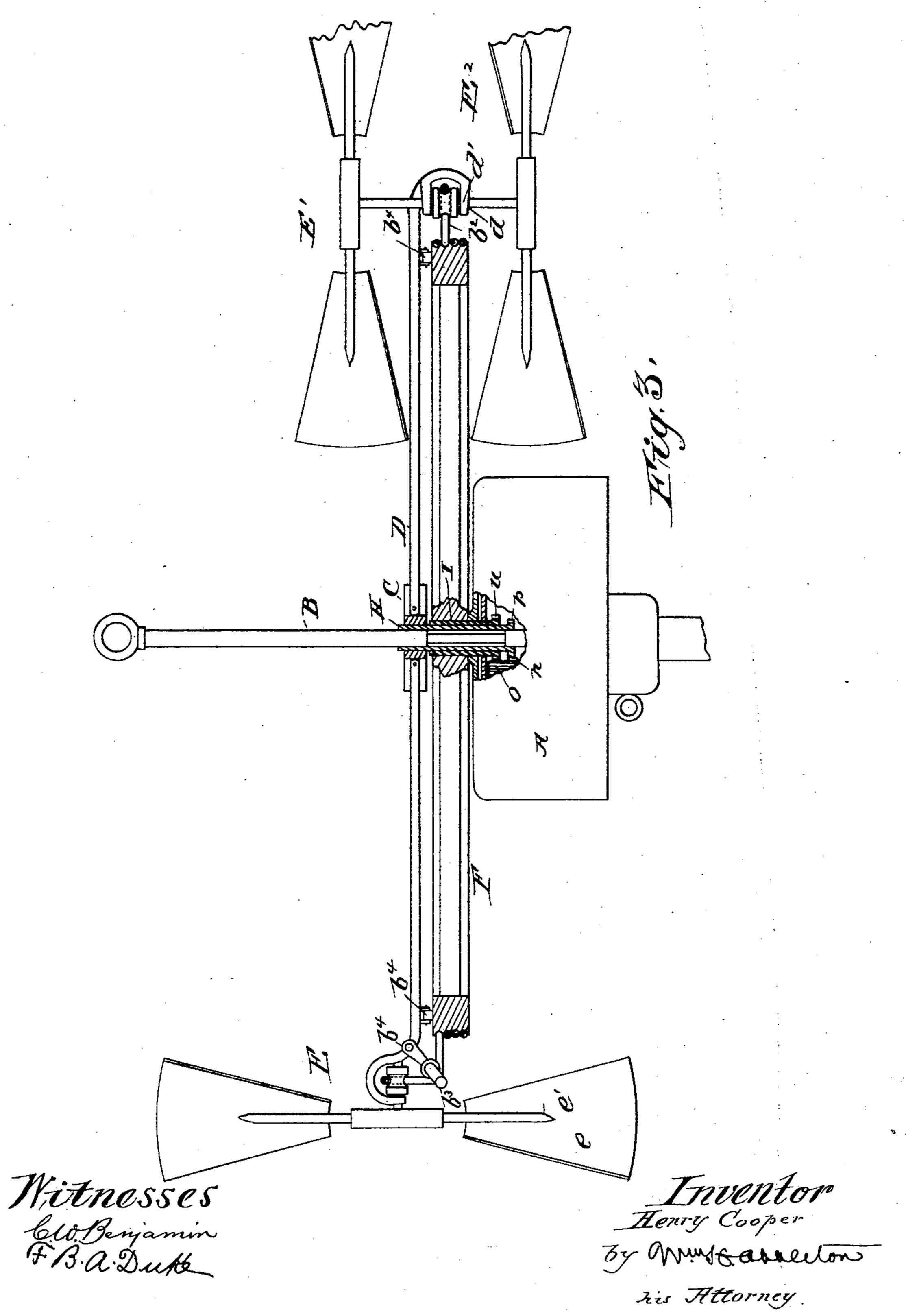
MACHINE FOR AGITATING AND CIRCULATING AIR IN ROOMS, &c. No. 455,660. Patented July 7, 1891.
