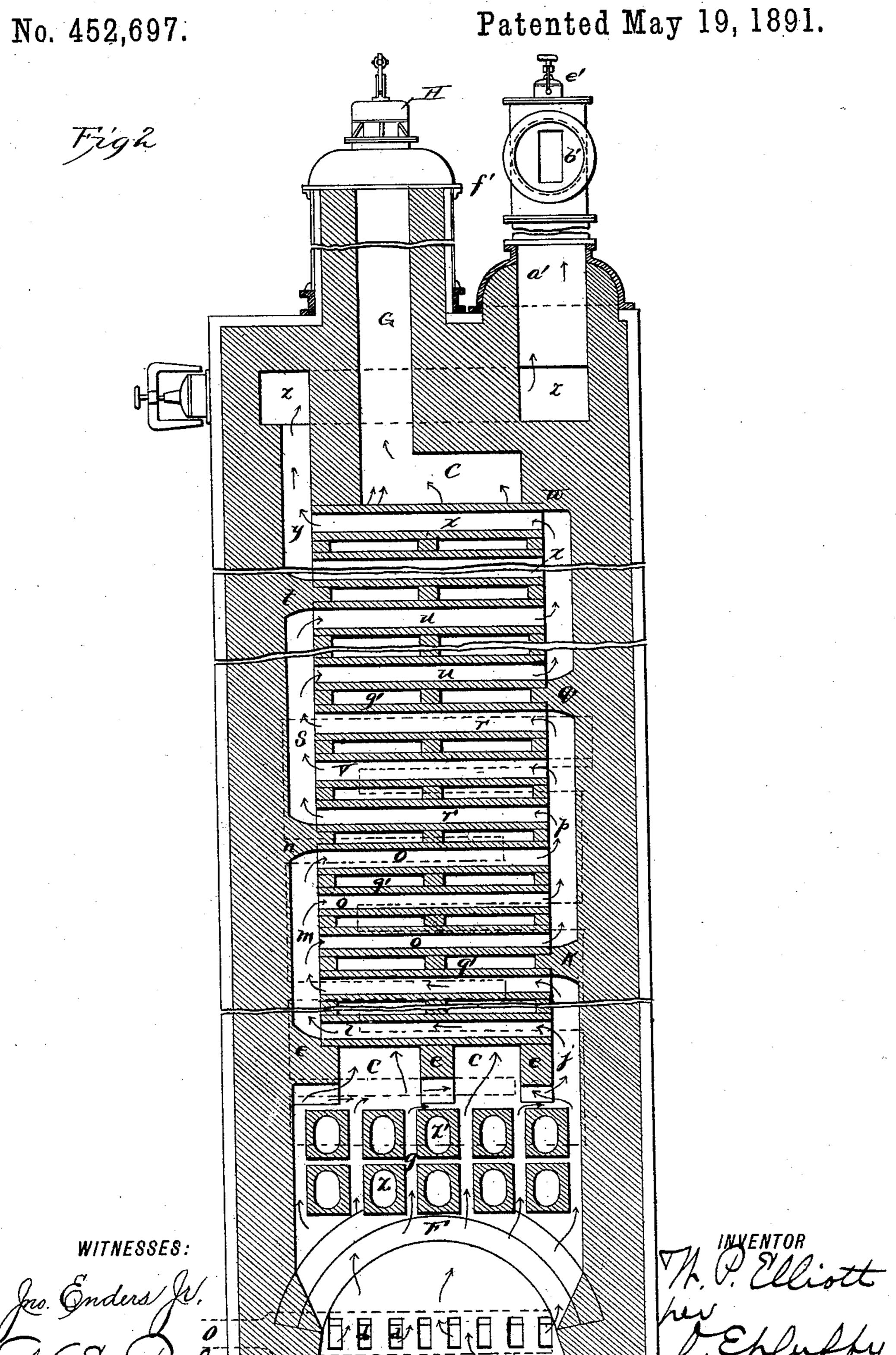
PROCESS OF AND APPARATUS FOR THE MANUFACTURE OF GAS.
