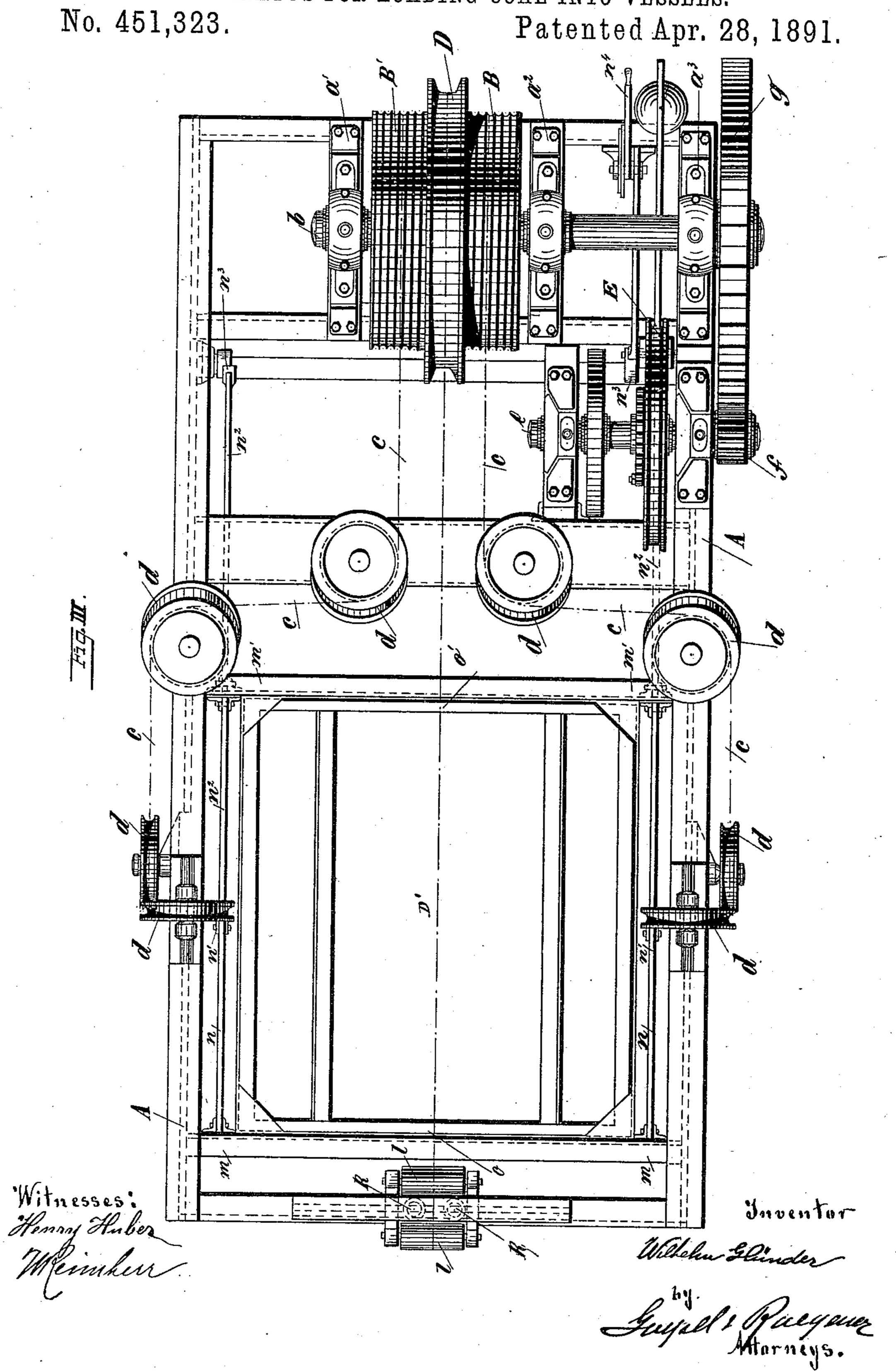
APPARATUS FOR LOADING COAL INTO VESSELS.
