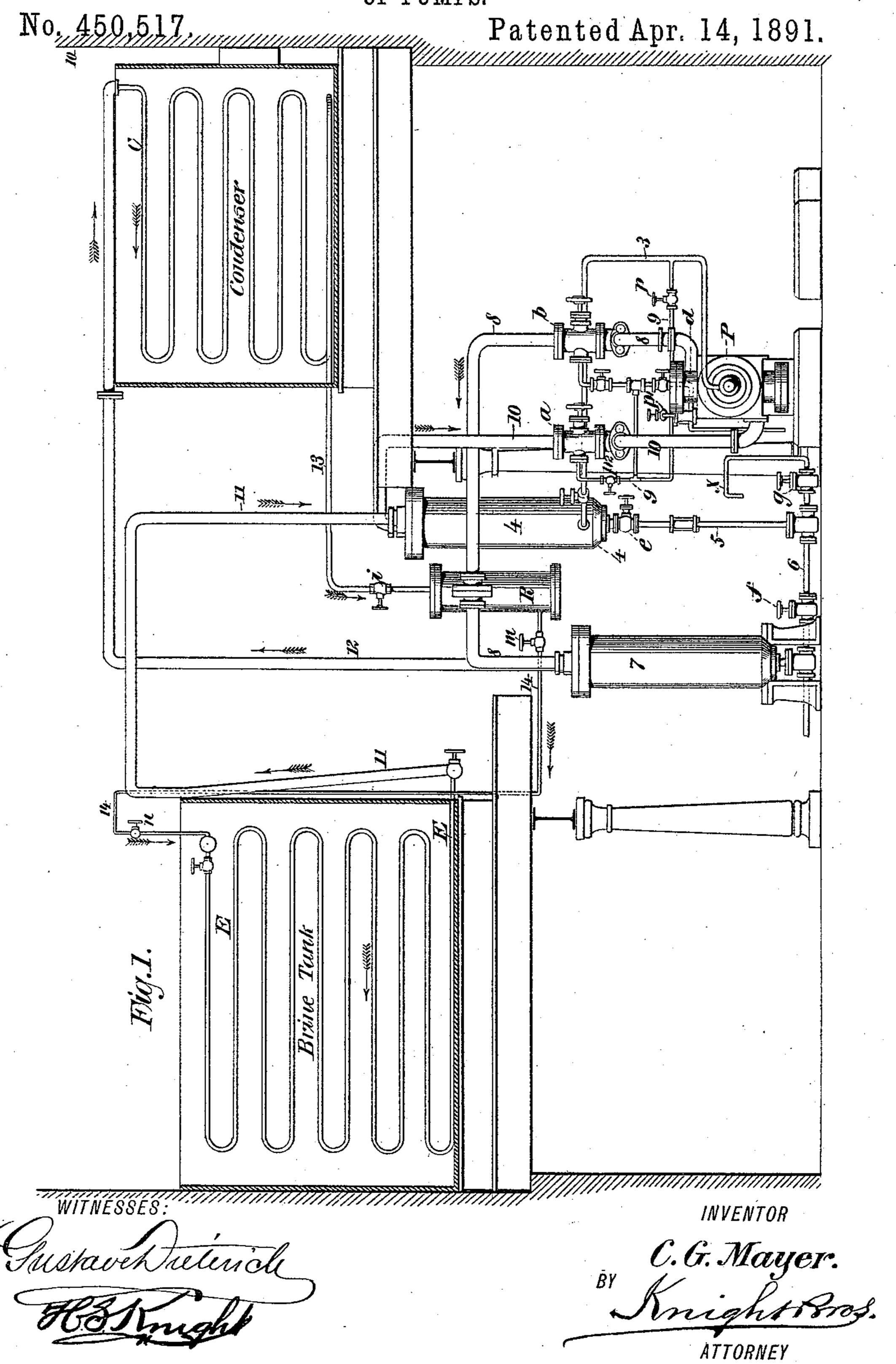
APPARATUS FOR COOLING AND LUBRICATING THE WORKING PARTS OF PUMPS.
