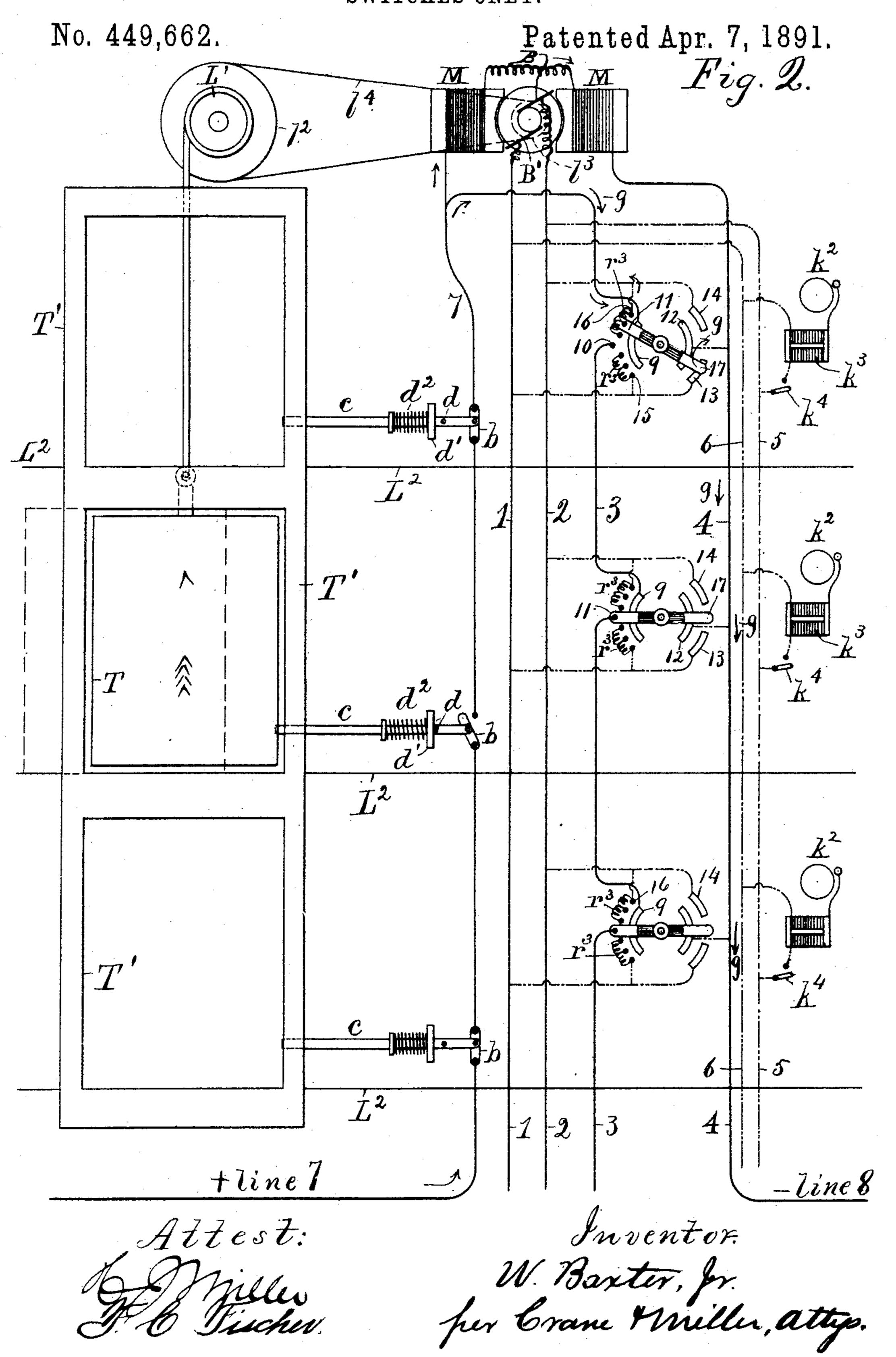
SYSTEM OF OPERATING ELECTRIC ELEVATORS WITH LANDING SWITCHES ONLY.
