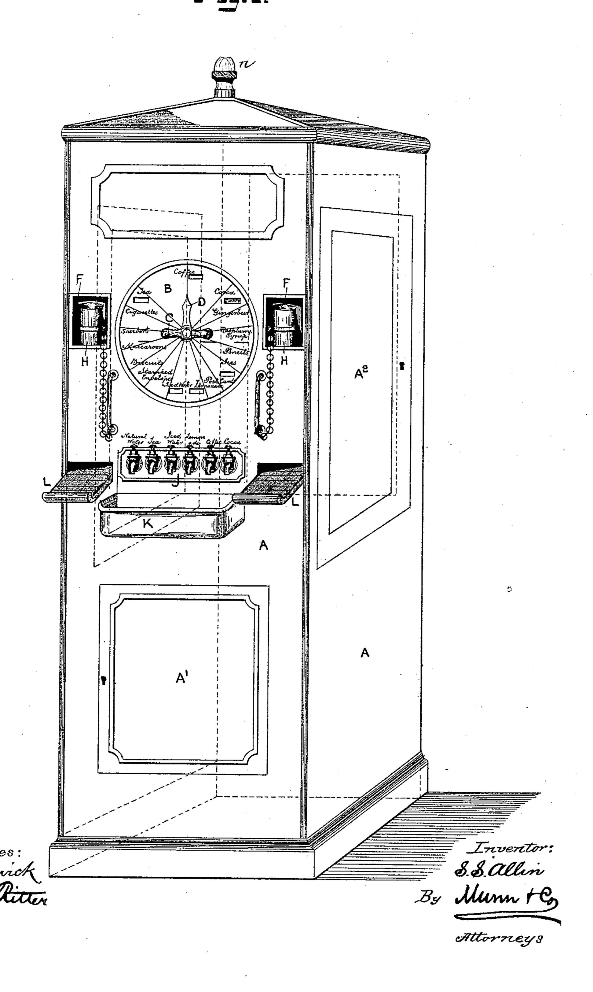
AUTOMATIC MACHINE FOR DELIVERING ARTICLES IN EXCHANGE FOR COIN.
