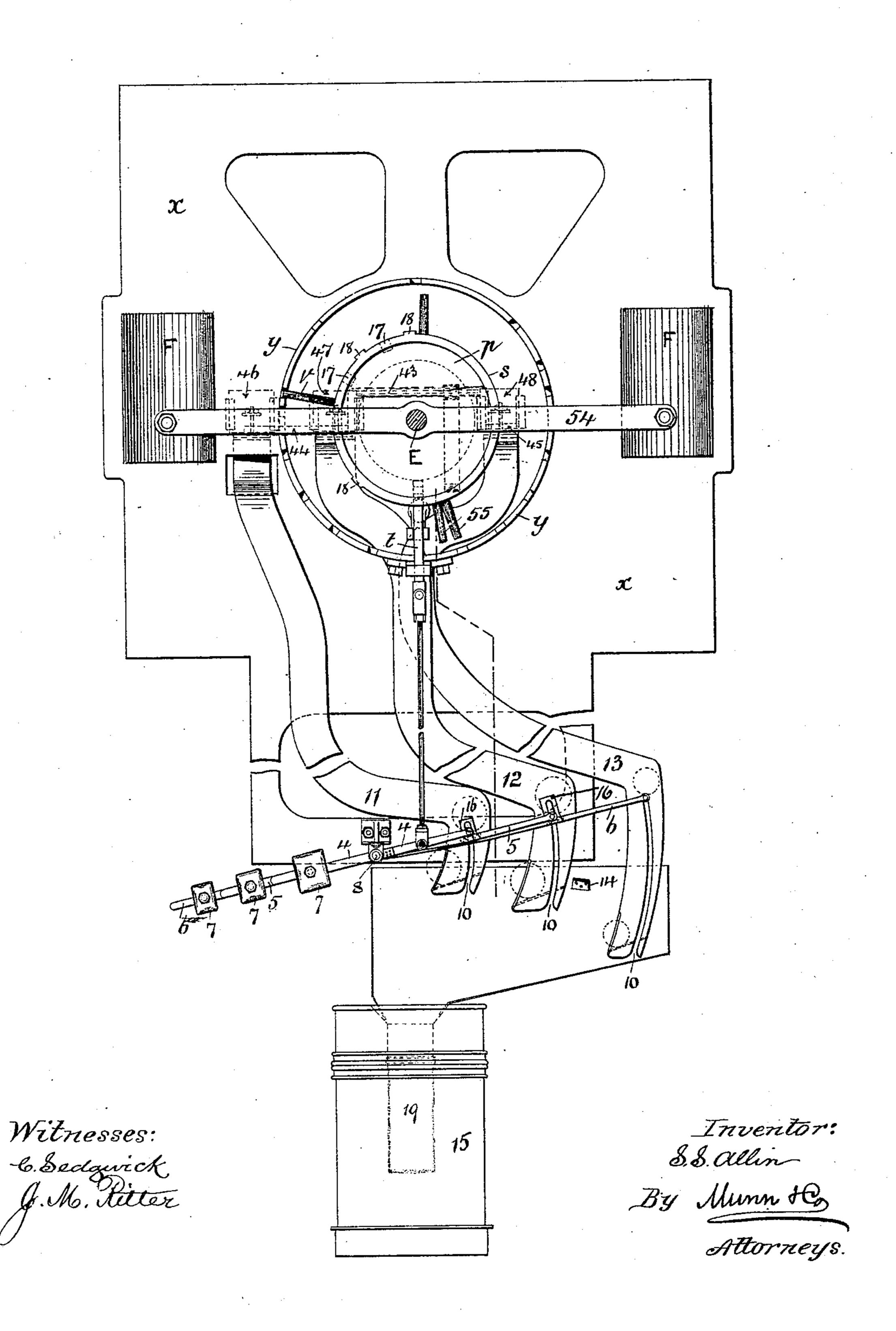
AUTOMATIC MACHINE FOR DELIVERING ARTICLES IN EXCHANGE FOR COIN.
