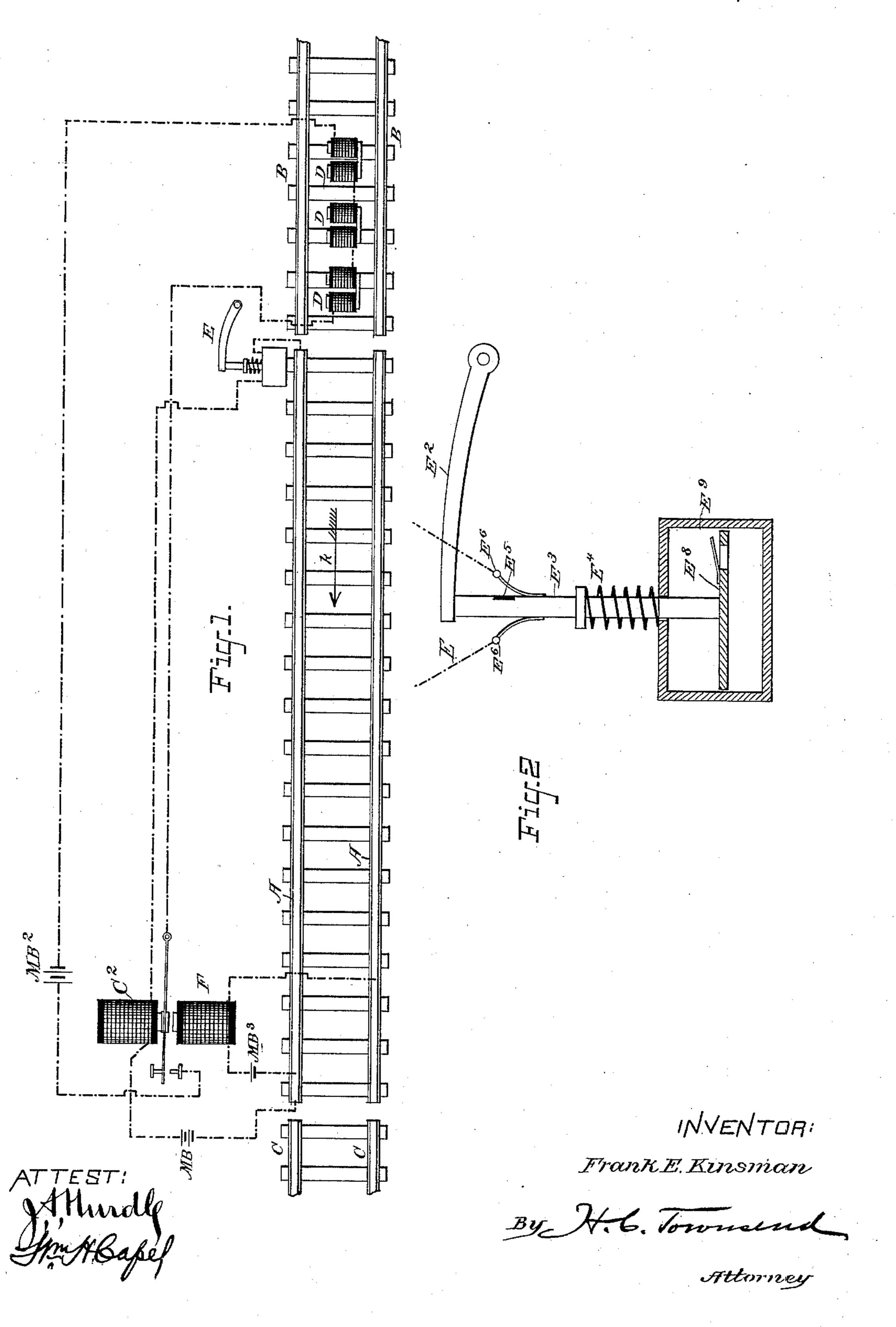
RAILWAY CIRCUIT FOR SIGNALING AND CONTROLLING TRAINS.
