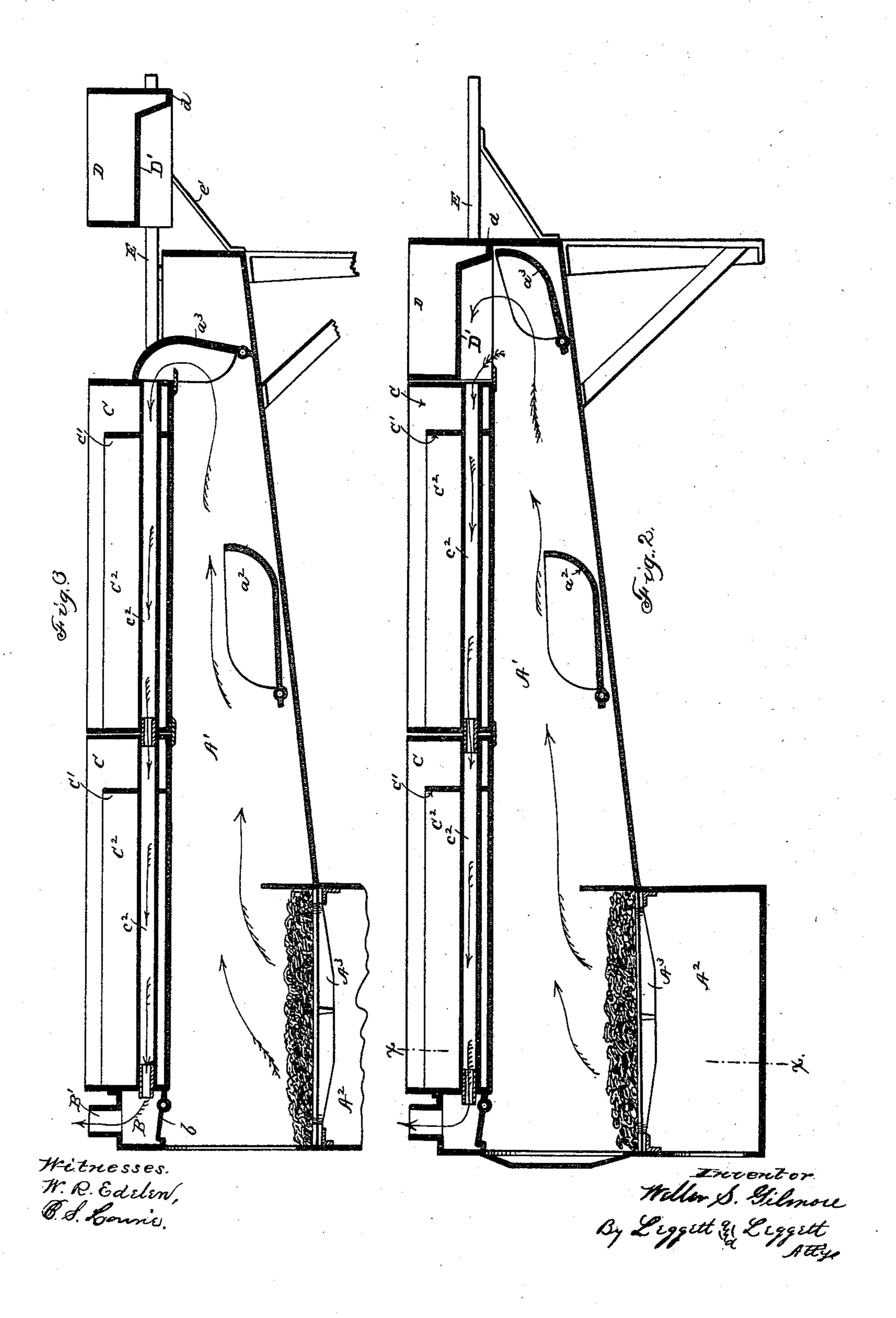
EVAPORATING PAN AND FURNACE FOR OPERATING THE SAME.
