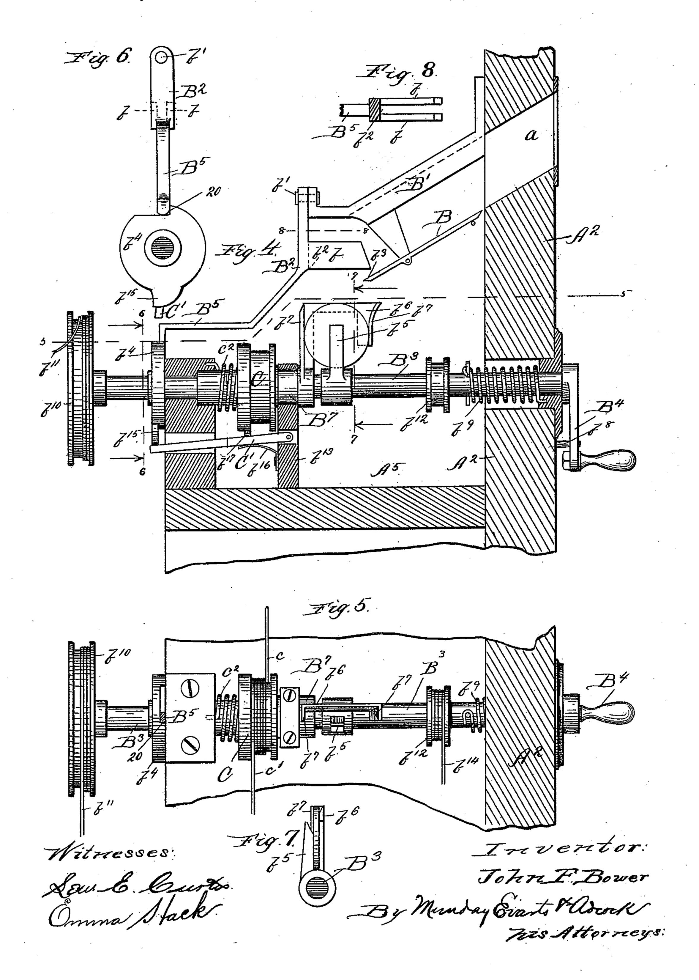
COIN CONTROLLED TESTING AND DISPLAY APPARATUS.
