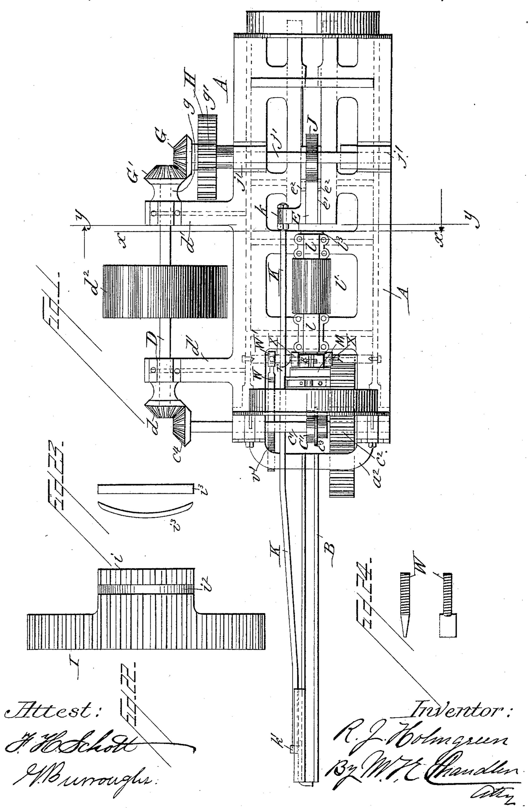
R. J. HOLMGREEN. MACHINE FOR TURNING BROOM HANDLES.
