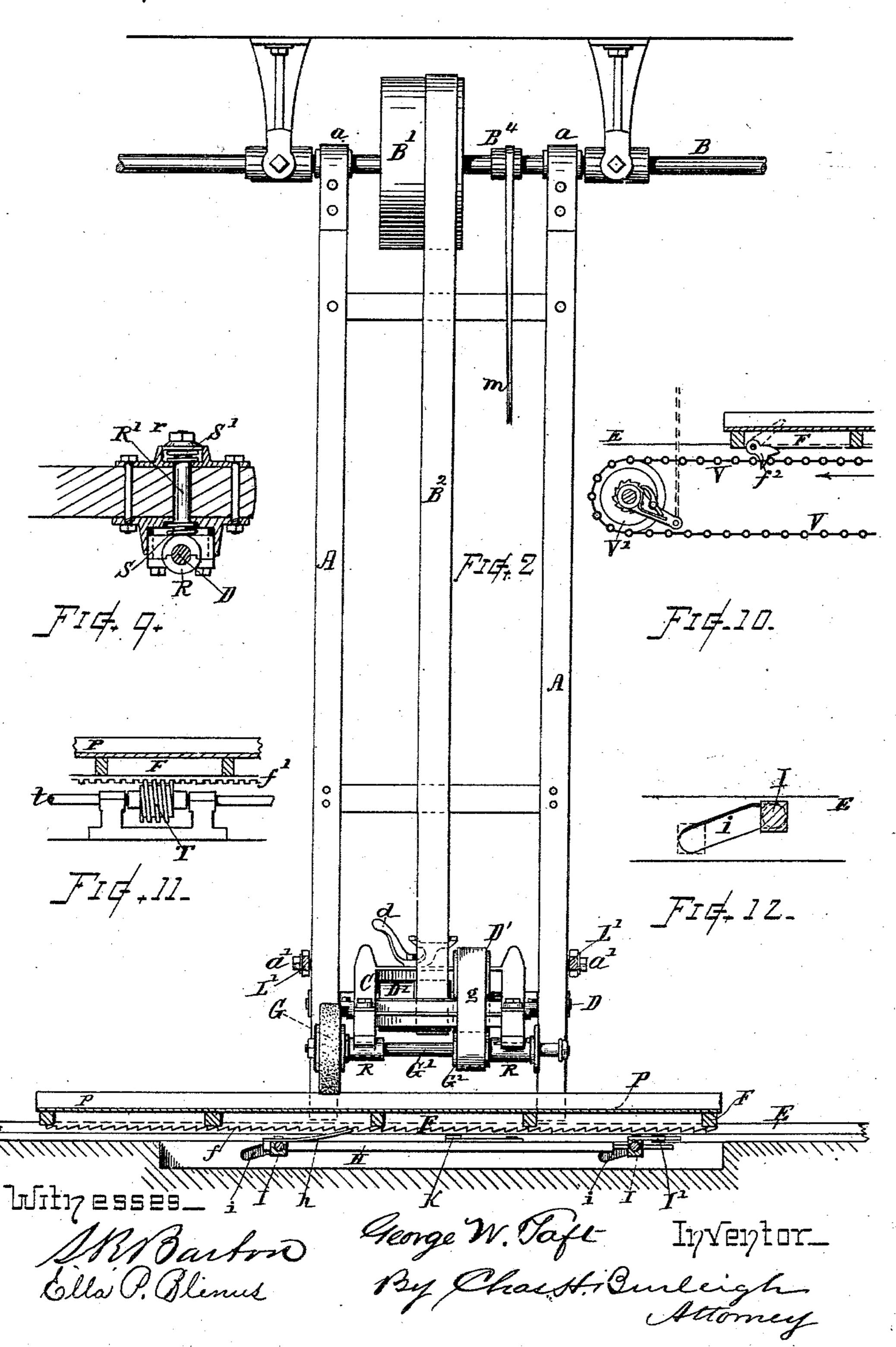
MACHINE FOR GRINDING AND POLISHING ROAD SCRAPER BLADES, &c. No. 411,839.
