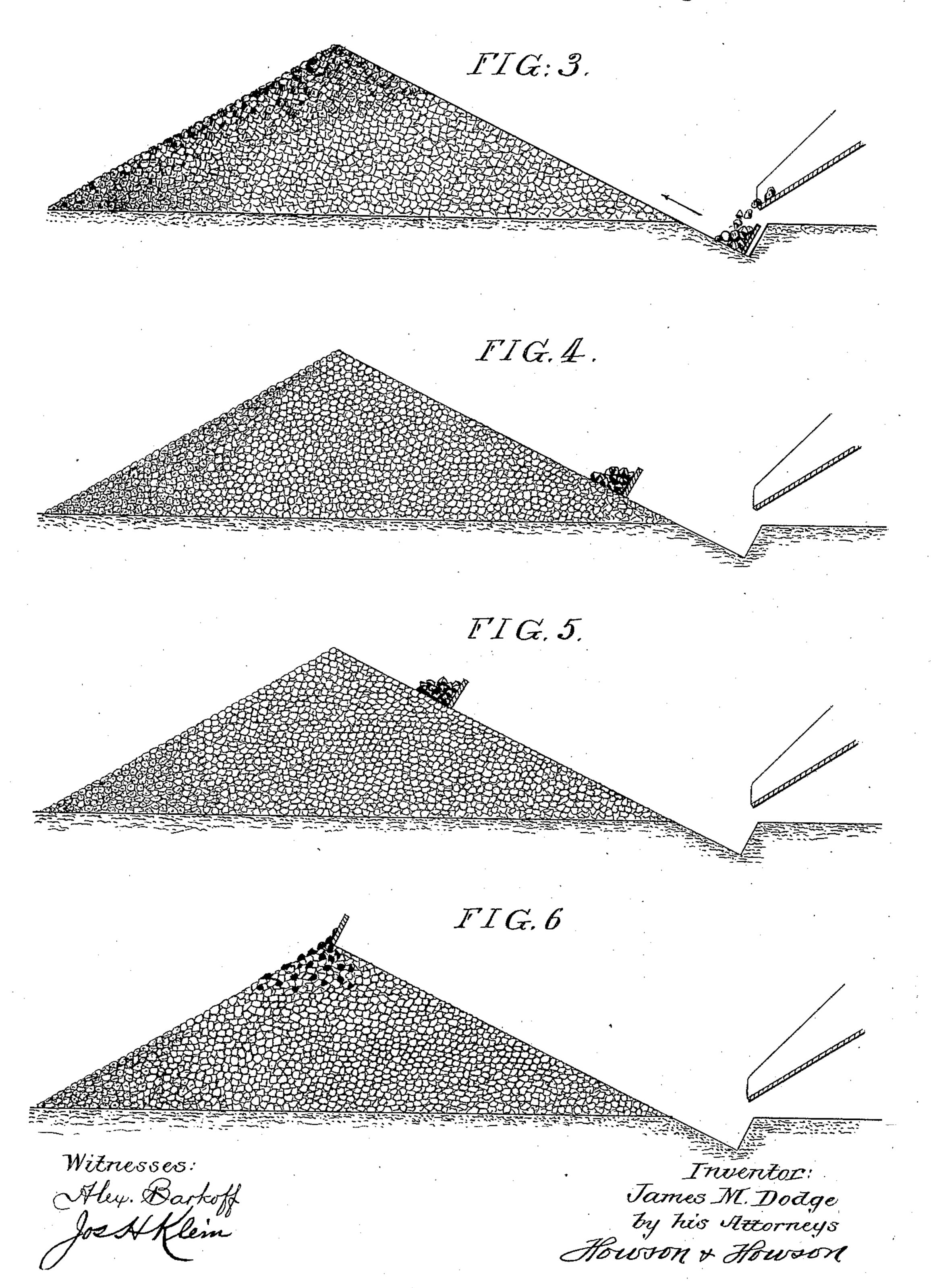
PROCESS OF PILING COAL OR ANALOGOUS MATERIAL.
