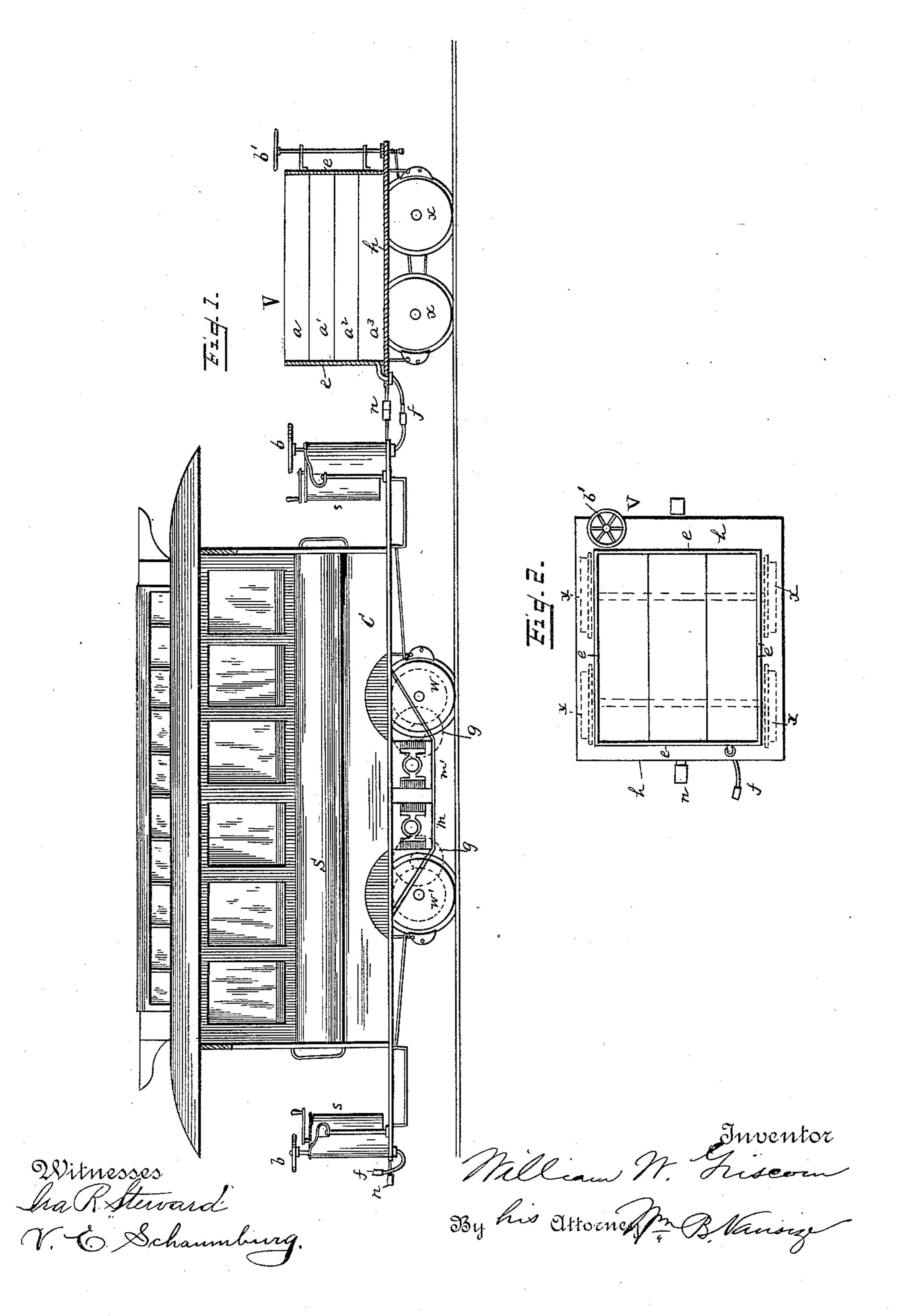
MEANS FOR PROPELLING VEHICLES BY SECONDARY BATTERIES.
