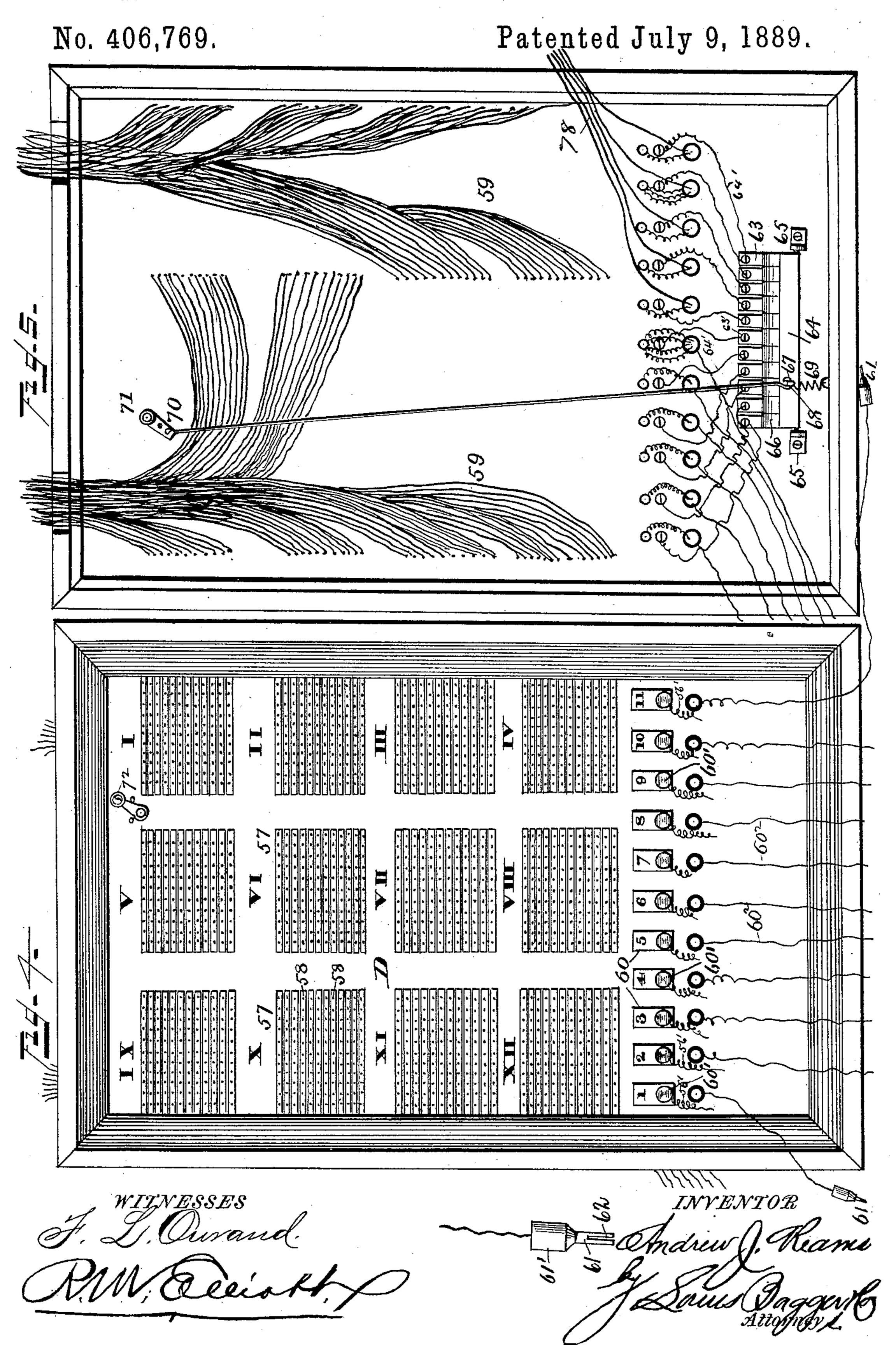
SIGNAL OR ALARM TRANSMITTER AND TIME INDICATOR.
