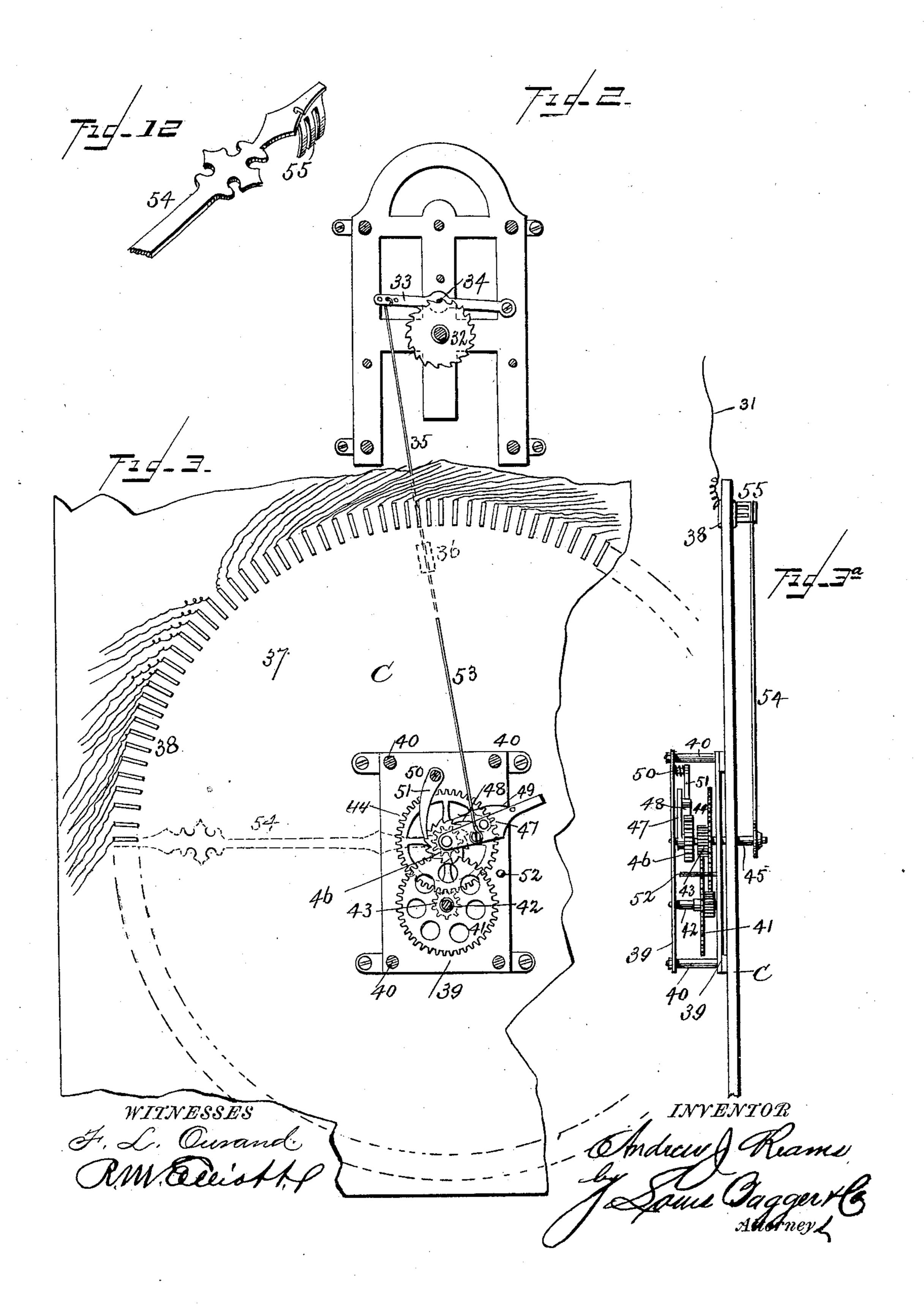
SIGNAL OR ALARM TRANSMITTER AND TIME INDICATOR.
