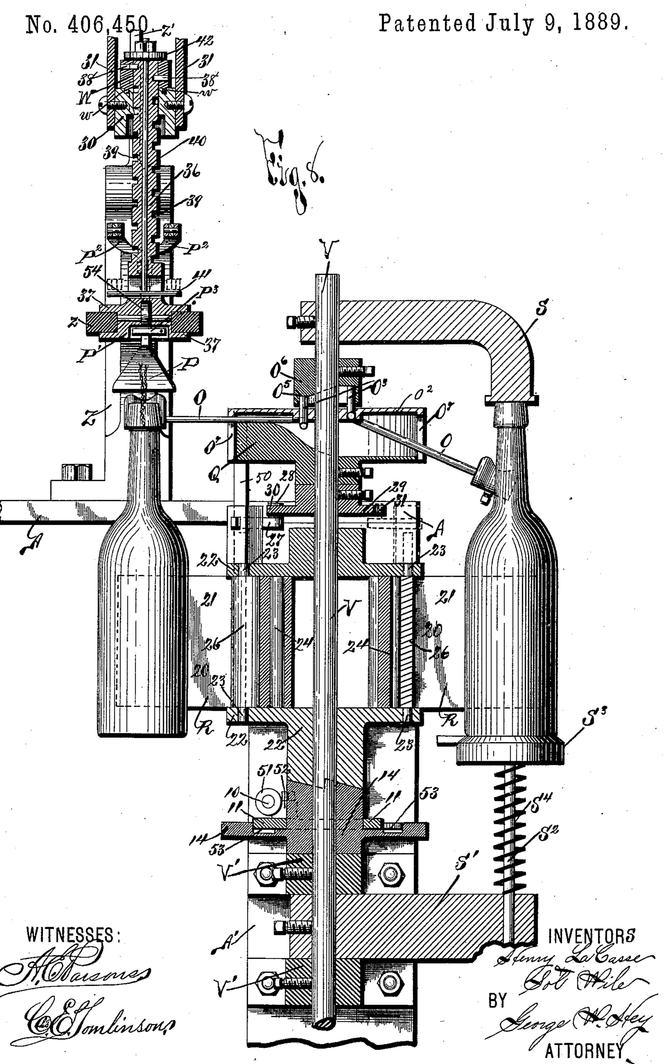
MACHINE FOR CORKING BOTTLES AND WIRING THE CORKS THERETO.
