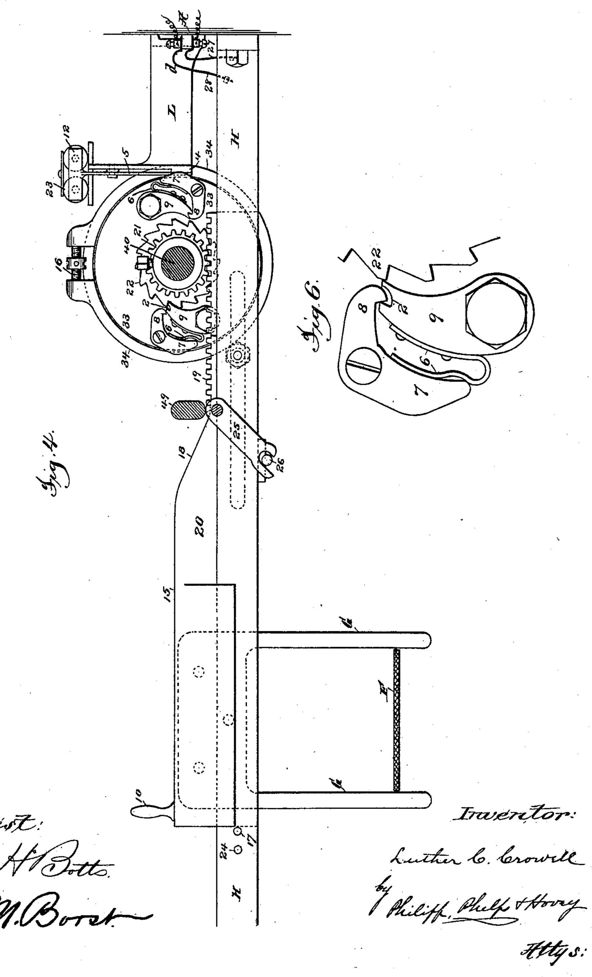
STOP MECHANISM FOR WEB PRINTING MACHINES.
