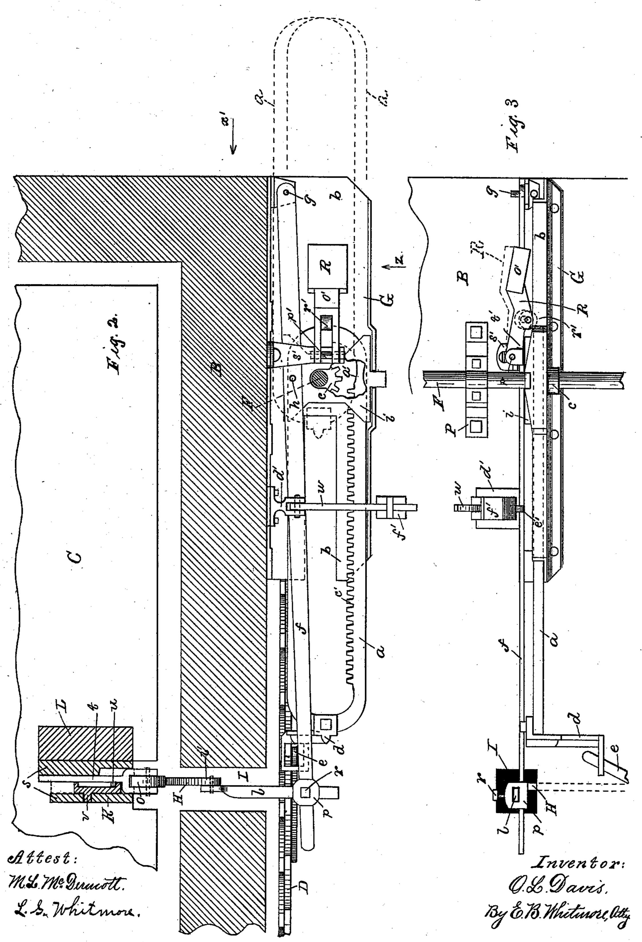
MECHANISM FOR OPERATING THE GATES OR DOORS OF ELEVATOR WELLS.
