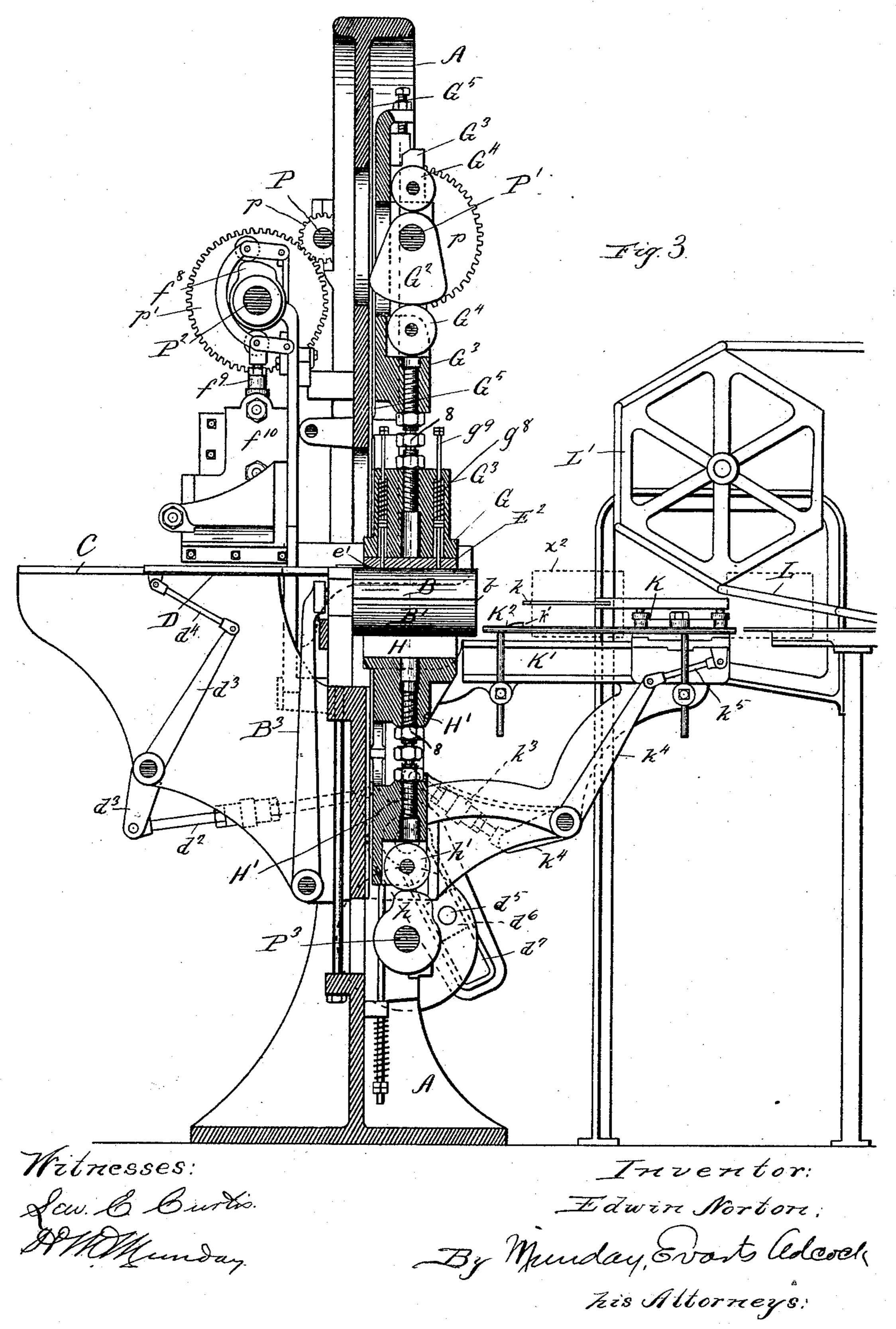
CAN FORMING AND SOLDERING MACHINE.
