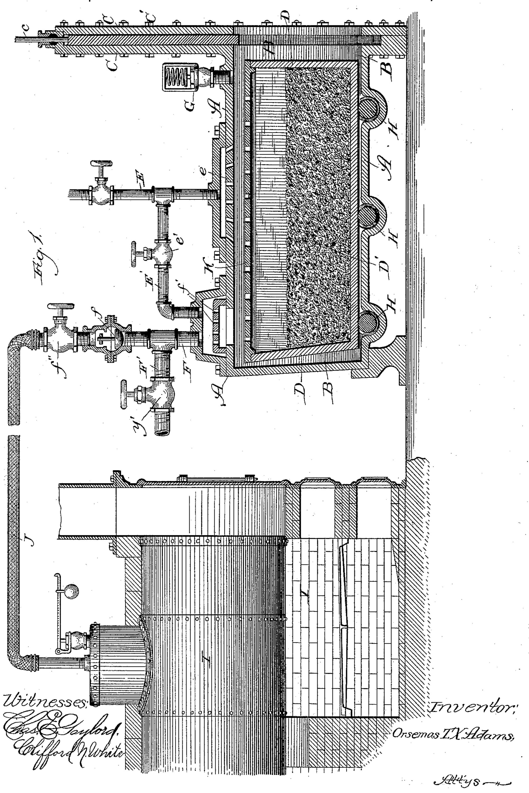
SMELTING FURNACE, SLAG STEAM GENERATING FURNACE AND PLANT.
