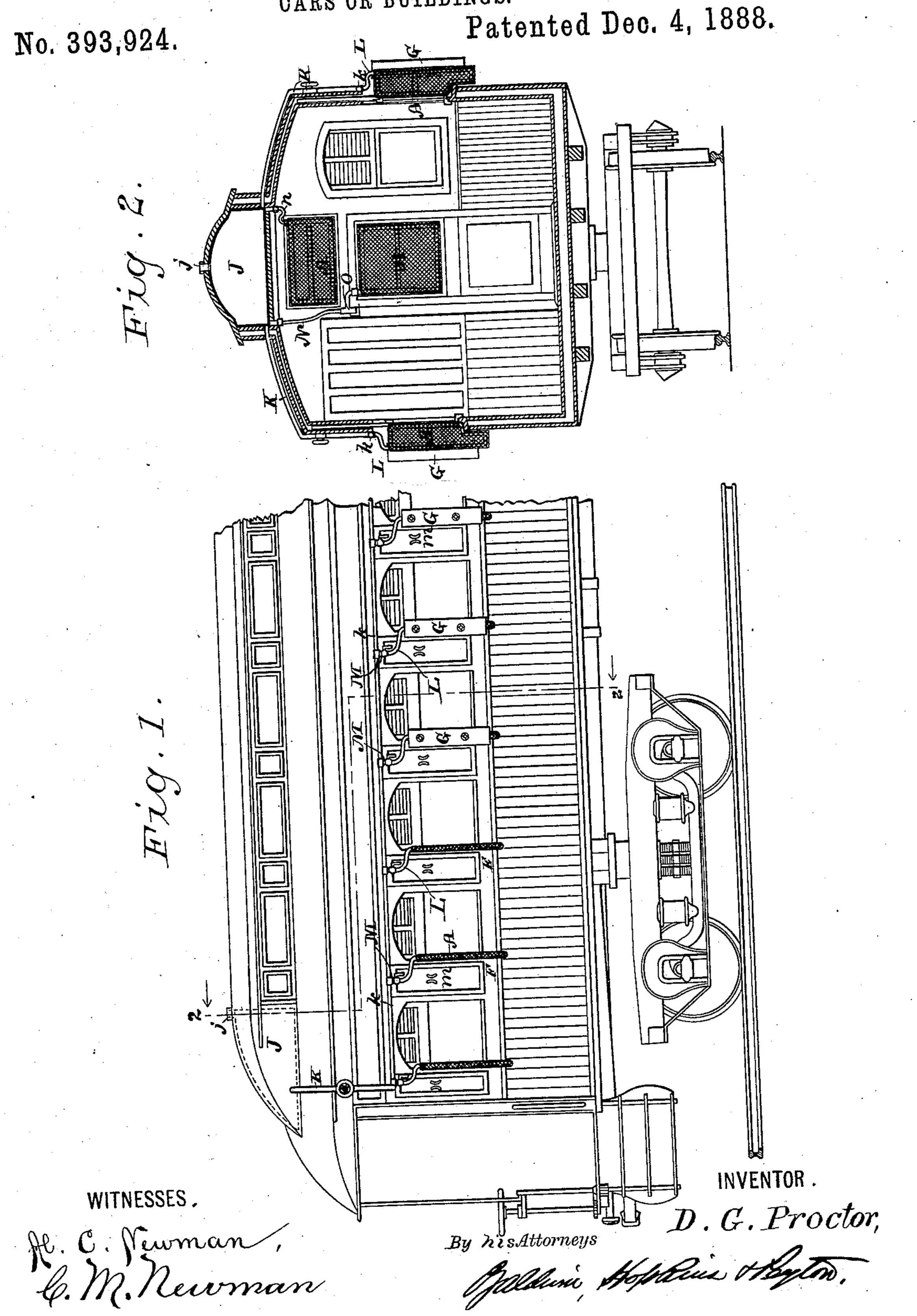
AIR PURIFYING, COOLING, AND VENTILATING DEVICE FOR RAILROAD CARS OR BUILDINGS.
