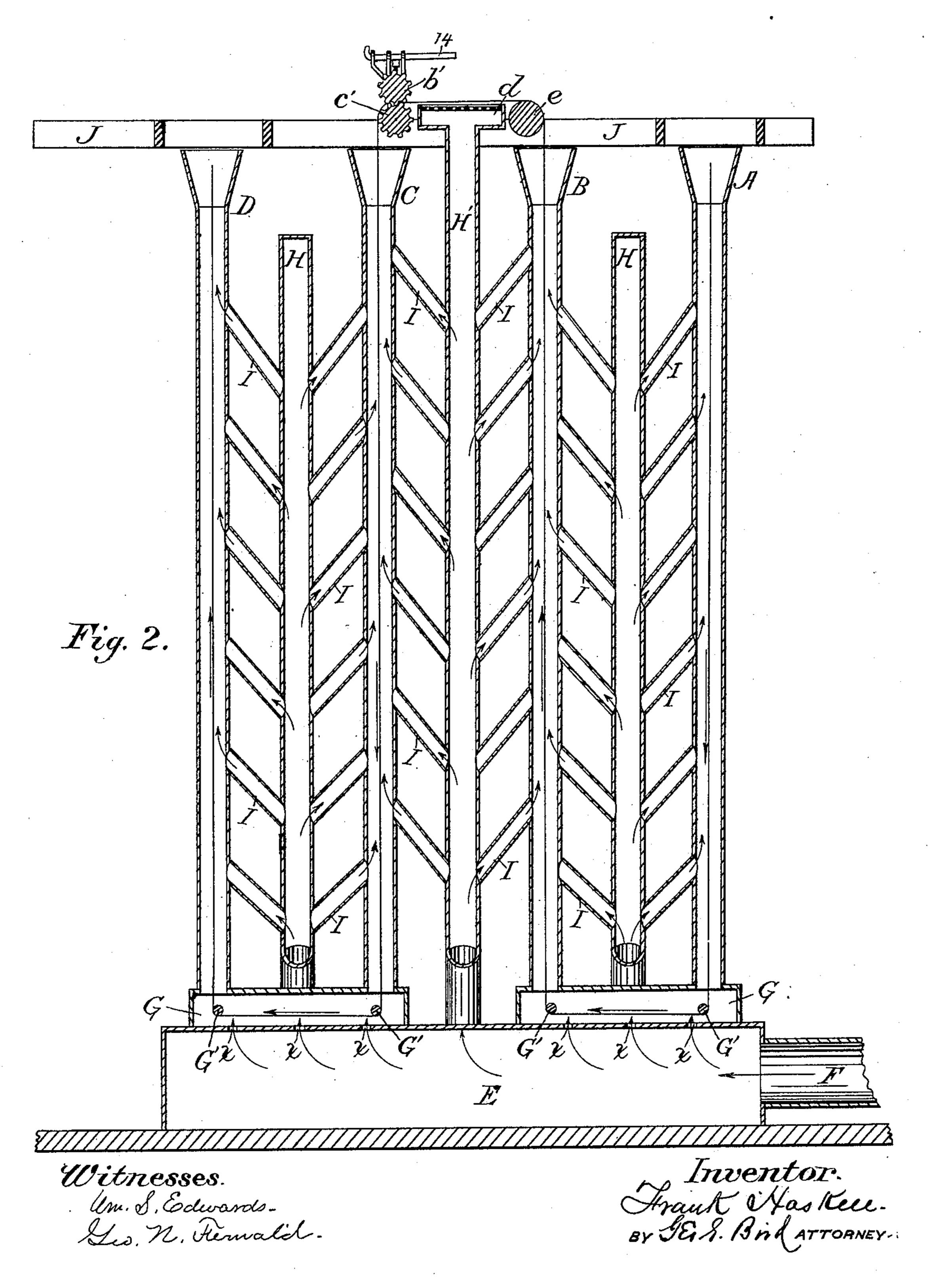
MACHINE FOR DRYING WARPS, &c.
