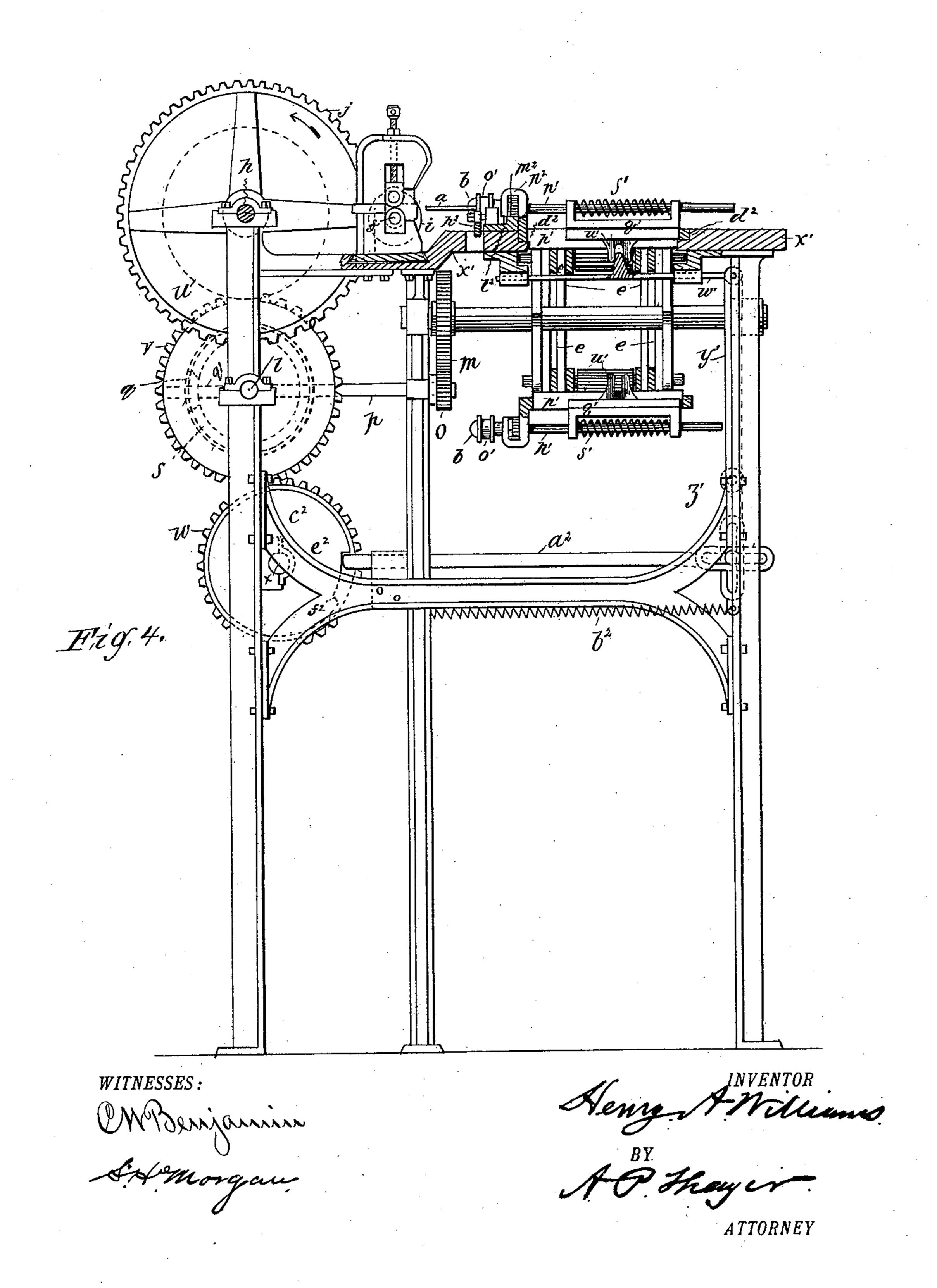
MACHINE FOR MAKING HACKLE PINS, AWLS, &c.
