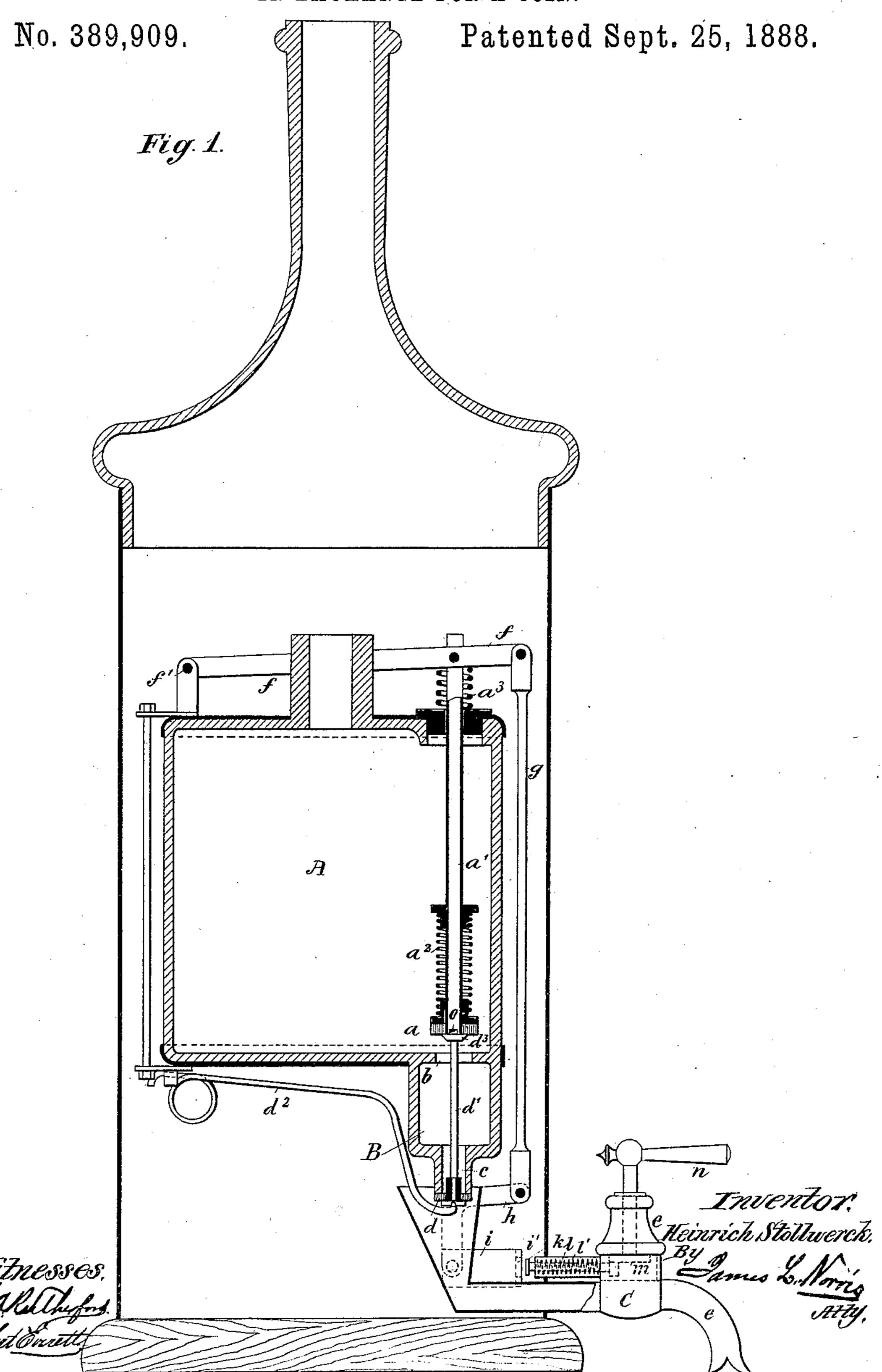
APPARATUS FOR THE DELIVERY OF A GIVEN QUANTITY OF LIQUID IN EXCHANGE FOR A COIN.
