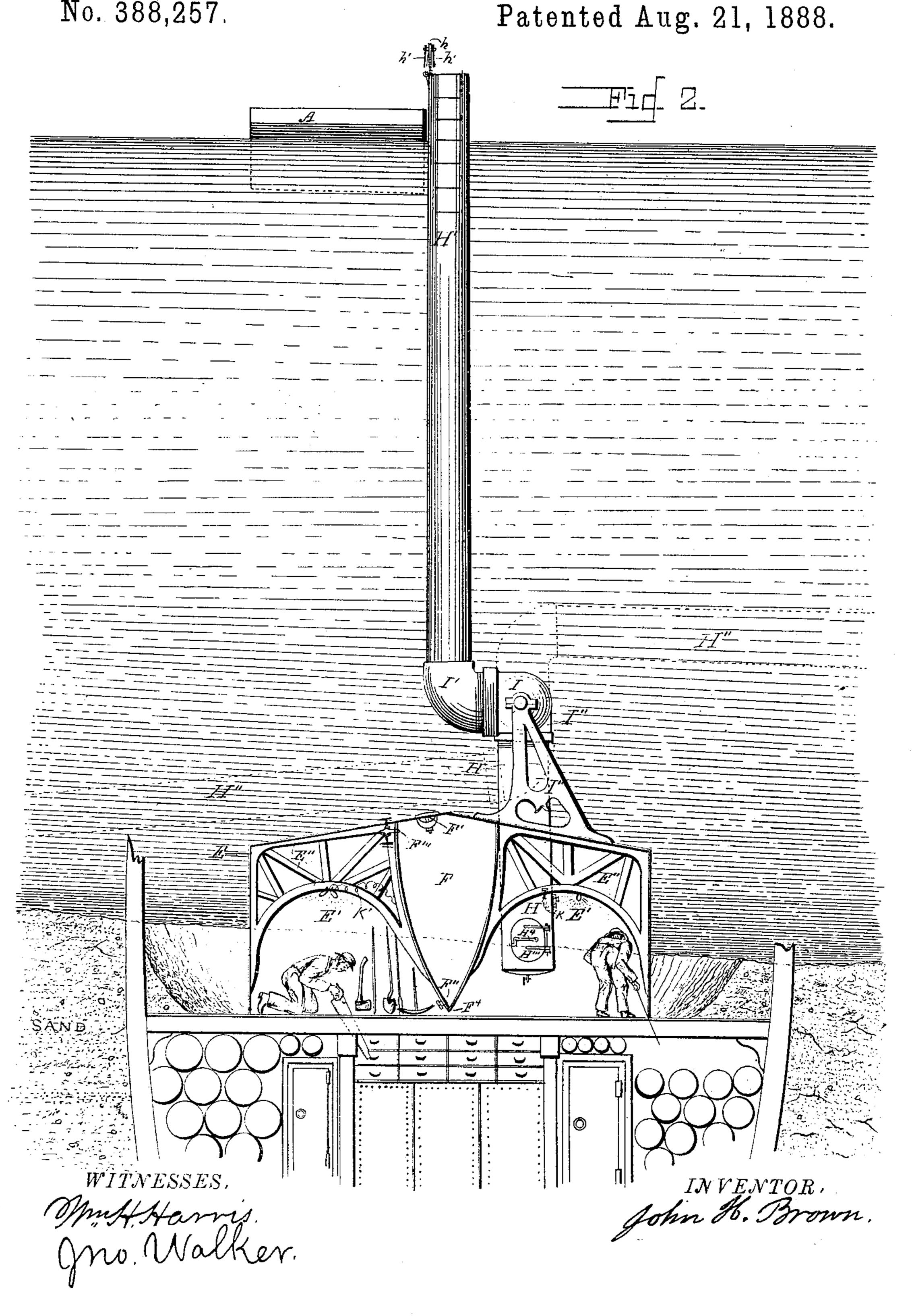
APPARATUS FOR RECOVERING VALUABLE CONTENTS FROM SUNKEN SHIPS.
