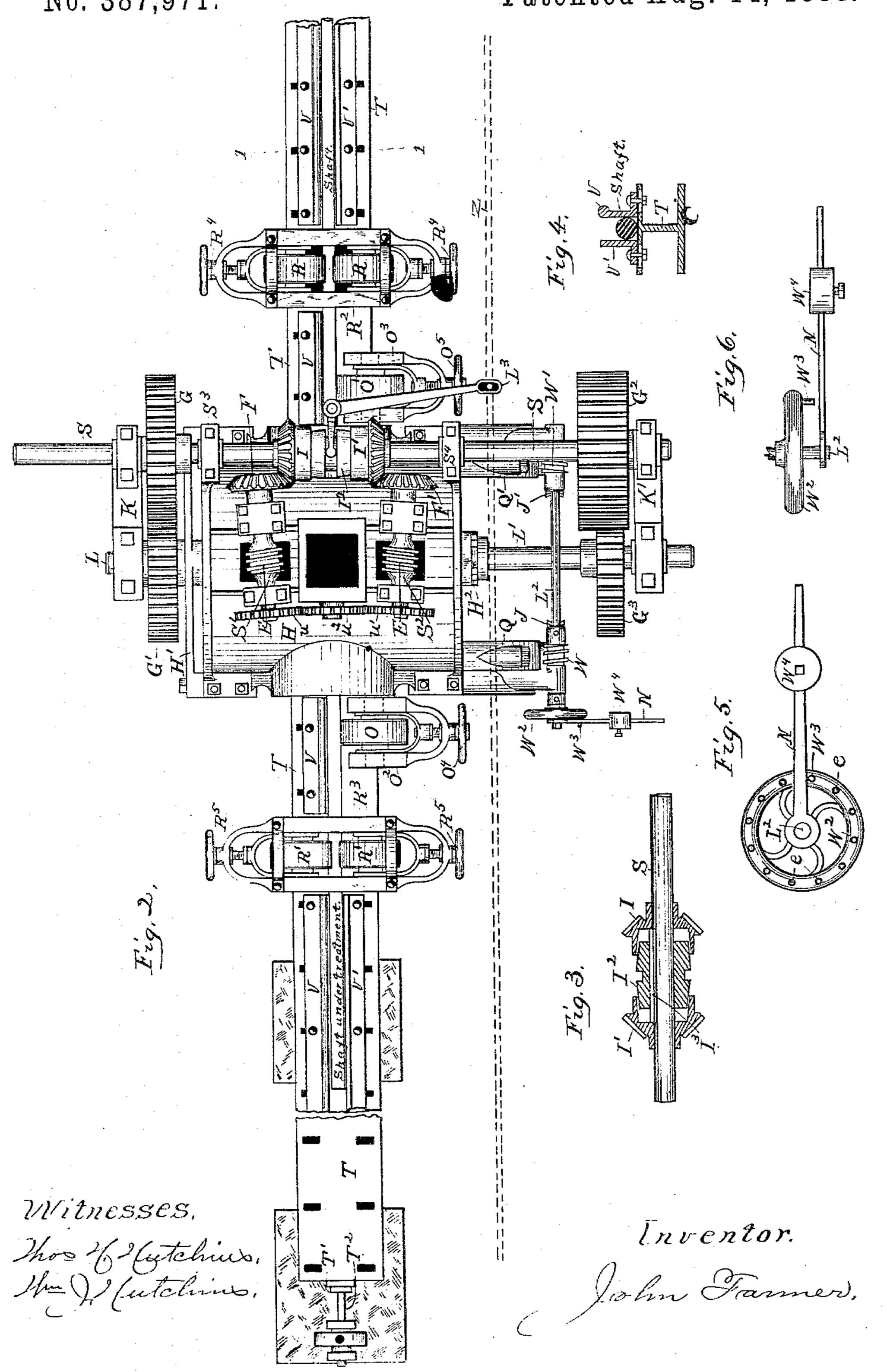
MACHINE FOR STRAIGHTENING, GRINDING, AND POLISHING METAL BARS.
